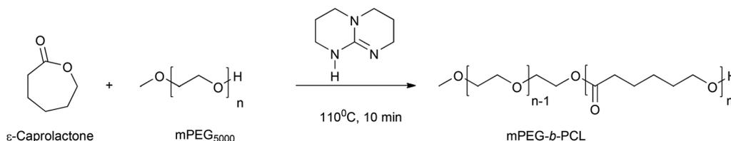
**Scheme 1** Schematic representation of the ring opening polymerization of (A)  $\delta$ -decalactone, (B)  $\omega$ -pentadecalactone and (C)  $\epsilon$ -caprolactone using different initiators to generate ranges of homopolymers and copolymers (RT-room temperature, TBD-1,5,7-triazabicyclo[4.4.0]dec-5-ene).
