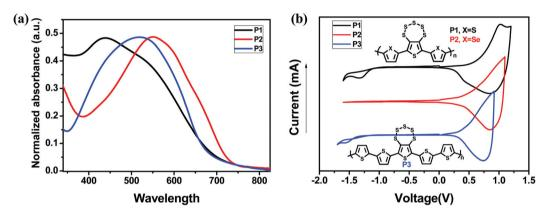
Fig. 4 (a) Absorption spectra of P1-P3 in thin film. (b) CV of P1, P2 and P3, using the DCM/TBAPF<sub>6</sub> solvent/electrolyte system.
