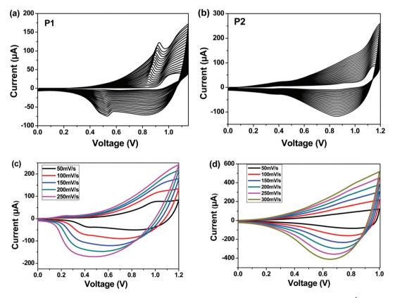
Fig. 3 (a) and (b) Multisweep electropolymerization of 2d and 2e on a Pt electrode in DCM and 0.1 M TBAPF<sub>6</sub> at 50 mV s<sup>-1</sup> vs. Ag/AgCl wire. (c) and (d) CV of P1 and P2 in monomer free DCM and 0.1 M TBAPF<sub>6</sub> as a function of scan rate.
