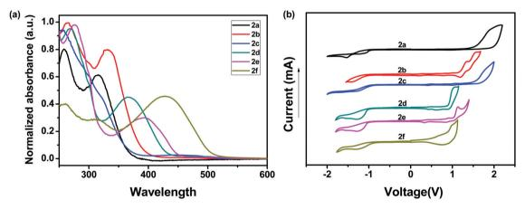
Fig. 2 (a) UV-vis spectra in DCM and (b) electrochemical properties of compounds 2a–2f in 0.1 M TBAPF<sub>6</sub> in dry DCM as the solvent using a Pt-disk working electrode, a Pt-wire counter electrode and a Ag/AgCl reference electrode.
