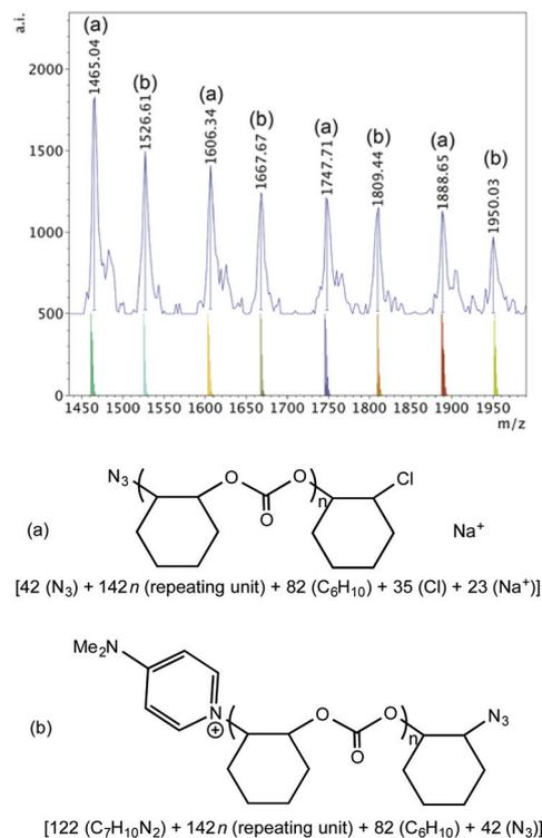
**Fig. 10** Lower mass region ( $m/z$  1400–2000,  $n = 9$ –12) of the MALDI-TOF mass spectrum produced by 1-DMAP according to Table 2, entry 11, with calculated masses of fragments shown beneath the observed spectrum and the proposed structures of polymers (a) and (b).
