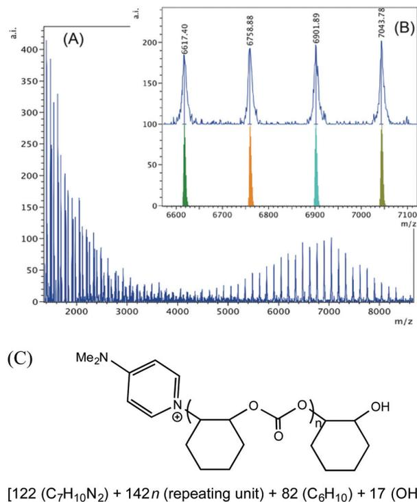
**Fig. 8** (A) MALDI-TOF mass spectrum of polycarbonate produced by 1·DMAP according to Table 2, entry 10. (B) Higher mass region ( $m/z$  6600–7100,  $n = 45$ –48) of the spectrum with calculated masses of fragments shown beneath the observed spectrum. (C) Proposed structure of the high mass range polymer.
