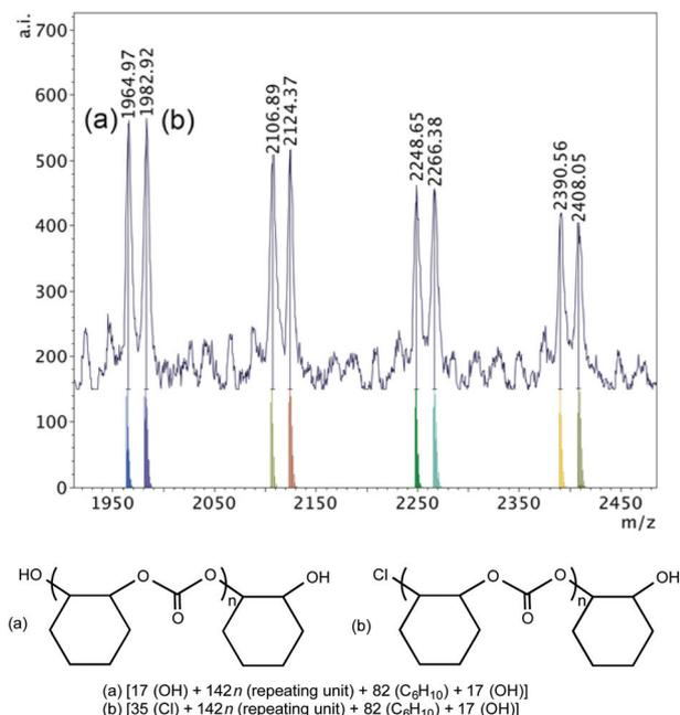
**Fig. 5** MALDI-TOF mass spectrum ( $m/z$  1950–2450,  $n = 13$ –17) produced by 1·DMAP according to Table 2, entry 7 with calculated masses of fragments shown beneath the observed spectrum and the proposed structures of polymers (a) and (b).
