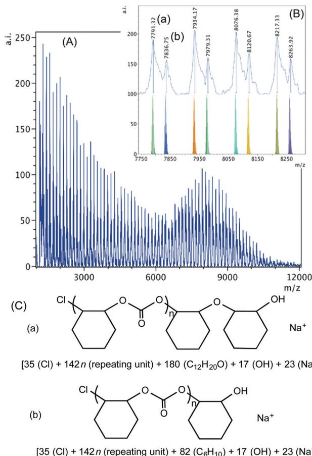
**Fig. 7** (A) MALDI-TOF mass spectrum produced by 1·THF according to Table 2, entry 5. (B) Higher mass region ( $m/z$  7750–8300,  $n = 53$ –56) of the spectrum with calculated masses of fragments shown beneath the observed spectrum. (C) Proposed structures of the high mass range polymers (a) and (b).
