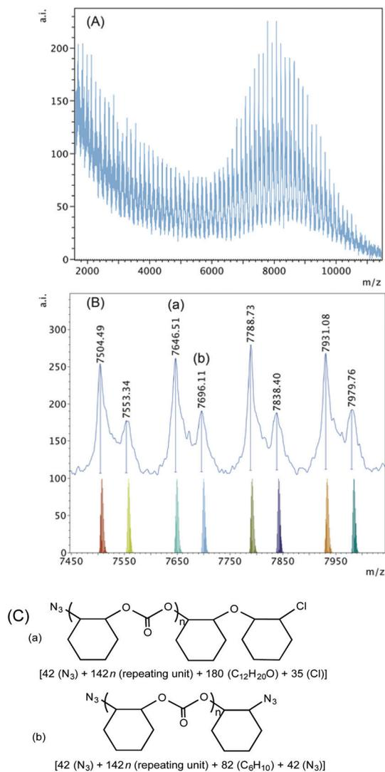
**Fig. 9** (A) MALDI-TOF mass spectrum produced by 1-THF according to Table 2, entry 6. (B) Higher mass region ( $m/z$  7450–8000,  $n = 51$ –54) of the spectrum with calculated masses of fragments shown beneath the observed spectrum. (C) Proposed structures of the high mass range polymers (a) and (b).
