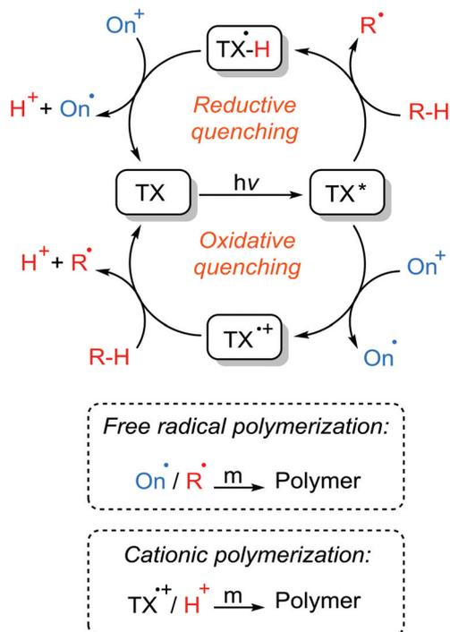
**Scheme 11** Three-component photoinitiation of free radical and/or cationic polymerizations in the presence of thioxanthone photosensitizer, amine hydrogen donor (R-H), and onium salt ( $\text{On}^+$ ) components: triplet thioxanthone is quenched through either oxidation by the onium salt or reduction by the amine hydrogen donor.
