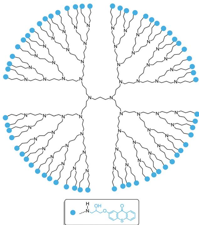
**Scheme 16** Dendritic poly(propylene imine) end-functionalized with thioxanthone moieties as a one-component *Type II* macrophotoinitiator.
