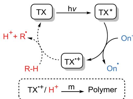
**Scheme 10** Photosensitized cationic polymerization using onium salts.
