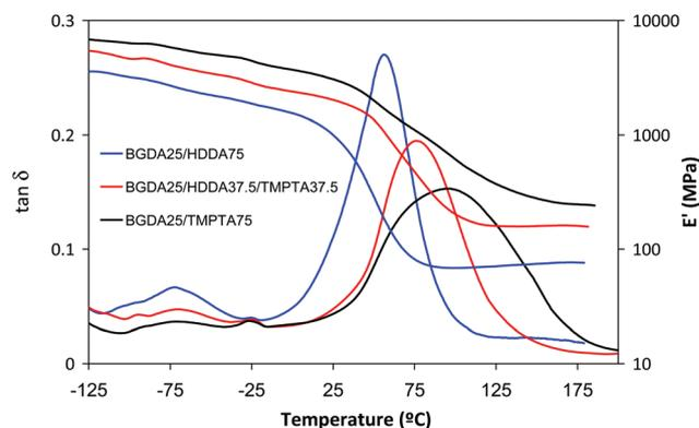
**Fig. 5** Storage moduli and  $\tan \delta$  curves against temperature of dual cured DETA 1 : 4 formulations with a 3 wt% of DMPA as a photoinitiator and different amounts of BGDA, HDDA and TMPTA, indicated in the legend.
