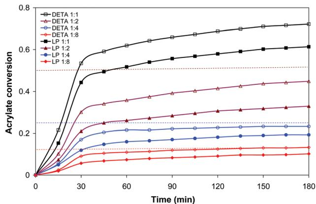
**Fig. 1** Acrylate conversion (from FTIR/ATR experiments) during aza-Michael addition (first curing stage) against time obtained by the isothermal reaction at 35 °C of BGDA25/HDDA75 formulations with a 3 wt% of DMPA as a photoinitiator and different molar ratios of LP and DETA, indicated in the legend. Horizontal dashed lines indicate the maximum acrylate conversion if aza-Michael addition would be completed for 1 : 8, 1 : 4 and 1 : 2 formulations.
