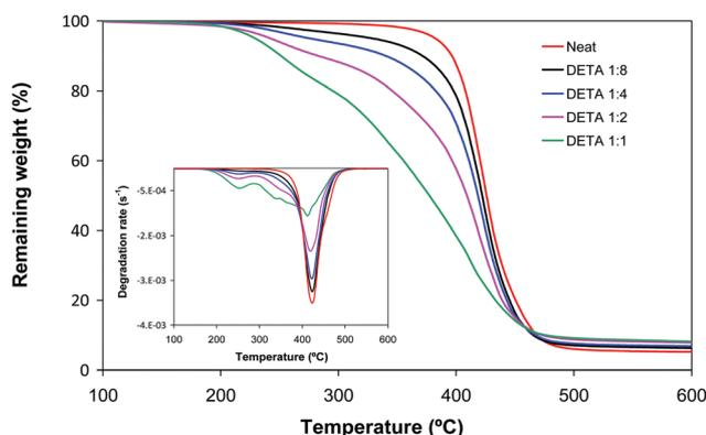
Fig. 4 Thermogravimetric curves at 10 °C min<sup>-1</sup> under a nitrogen atmosphere of dual cured BGDA25/HDDA75 formulations with a 3 wt% of DMPA as a photoinitiator and different molar ratios of DETA/acrylate, indicated in the legend.
