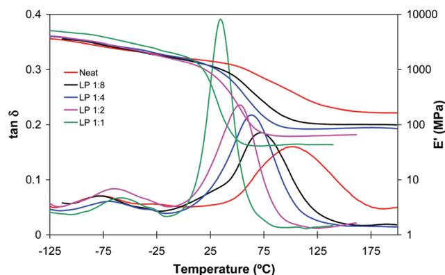
**Fig. 2** Storage moduli and  $\tan \delta$  curves against temperature of dual cured BGDA25/HDDA75 formulations with a 3 wt% of DMPA as a photoinitiator and different molar ratios of LP/acrylate, indicated in the legend.
