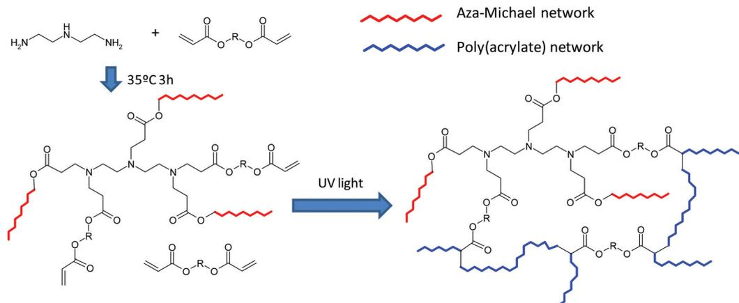
Scheme 1 Methodology for dual-network formation from amine-acrylate mixtures.
