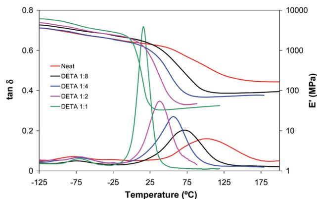
**Fig. 3** Storage moduli and  $\tan \delta$  curves against temperature of dual cured BGDA25/HDDA75 formulations with a 3 wt% of DMPA as a photoinitiator and different molar ratios of DETA/acrylate, indicated in the legend.
