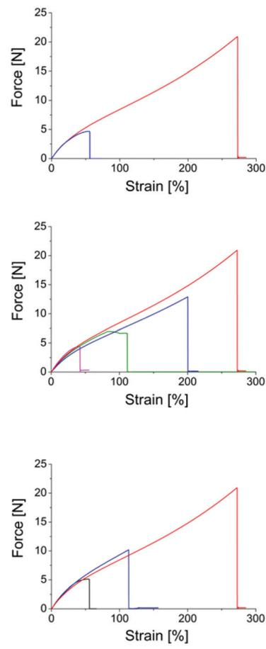
**Fig. 7** Lap shear tests on cured rubbers: (a) comparison between DA- (blue) and DTDB- (red) cured rubbers, adhesion for 30 min at 180 °C, (b) DTDB-cured rubber adhered at 180 °C for varying times (pink: 5 min, green: 10 min, blue: 20 min and red: 30 min), (c) DTDB-cured rubber adhered for 30 min at different temperatures (black: 100 °C, blue: 150 °C and red: 180 °C).
