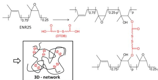
**Fig. 1** Crosslinking of ENR25 (25 mol% epoxidized): schematic representation of the disulfide containing network. The ratio of the epoxy function per diacid molecule is fixed at 25 to provide the network with optimal mechanical properties.<sup>31</sup>
