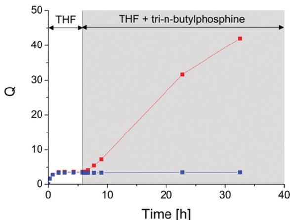
Fig. 3 Reductive swelling experiment (red: DTDB-cured sample, blue: DA-cured sample). The reductive agent was introduced after 6 hour equilibration in pure THF.
