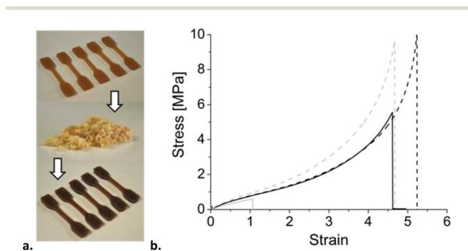
**Fig. 8** Recycling experiment. (a) The cured rubber is finely ground and then reshaped by compression moulding. (b) Tensile test before and after the recycling experiment (black: DTDB-cured; grey: DA-cured; dashed: before; line: after).
