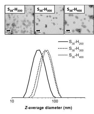
Fig. 5 TEM images and corresponding DLS particle size distributions obtained for spherical  $S_{38}$ - $H_x$ -10 nanoparticles when x = 200, 300 or
