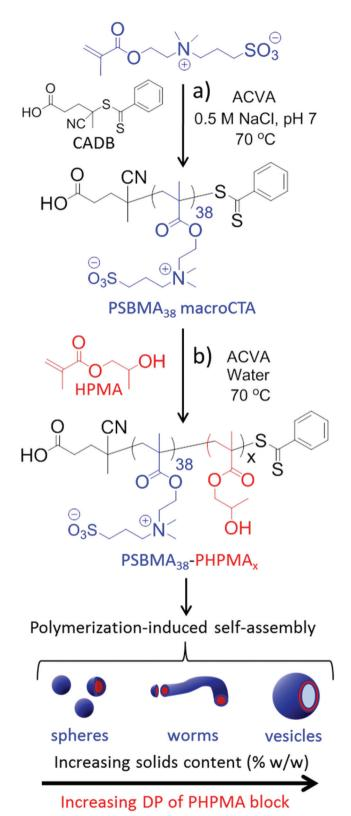
Fig. 1 (a) Synthesis of the PSBMA<sub>38</sub> macro-CTA via RAFT aqueous solution polymerization of SBMA. (b) RAFT aqueous dispersion polymerization of HPMA using this PSBMA<sub>38</sub> macro-CTA at 70 °C to afford various PSBMA-PHPMA diblock copolymer nano-objects via polymerizationinduced self-assembly (PISA).
