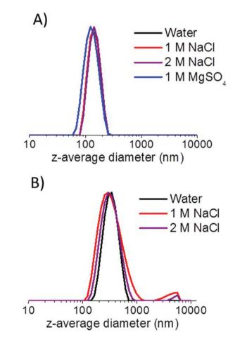
Fig. 10 Intensity-average particle size distributions obtained by DLS for (a)  $S_{38}$ - $H_{400}$  vesicles and (b)  $G_{71}$ - $H_{400}$  vesicles after being aged in various aqueous salt solutions for one week.
