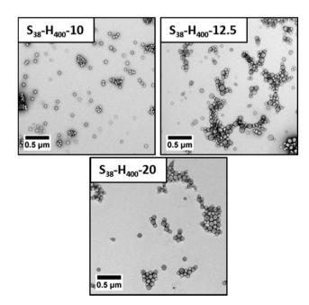
Fig. 6 Representative TEM images obtained for PSBMA<sub>38</sub>-PHPMA<sub>400</sub> nanoparticles prepared at various solids contents. The copolymer morphology evolves from kinetically-trapped spheres (10% w/w) to equilibrium vesicles (20% w/w) via a spheres plus vesicles mixed phase (12.5% w/w).
