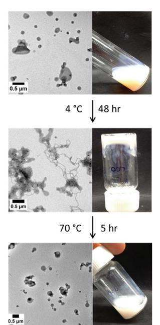
Fig. 9 TEM images and physical state of the dispersions obtained for (top)  $S_{38}$ - $H_{310}$ -25 vesicles at 20 °C and (middle) a mixed phase of worms and vesicles formed after being held at 4 °C for 48 h and (bottom) a mixed phase of vesicles and short worms obtained after heating to 70 °C for 5 hours.
