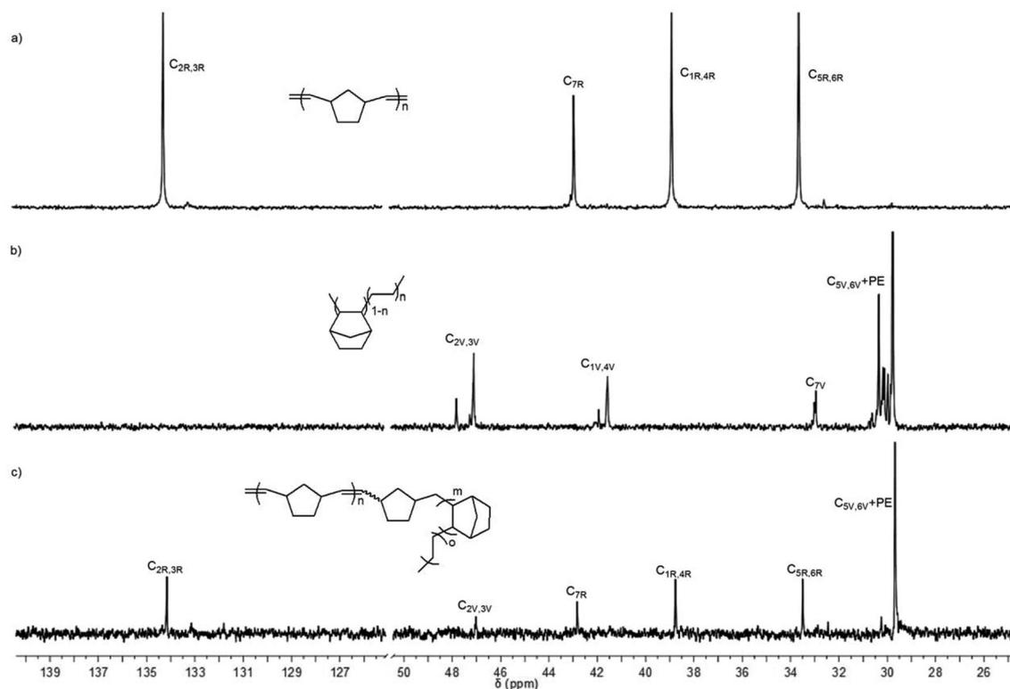
Fig. 6 <sup>13</sup>C NMR spectra of (a) poly(NBE)<sub>ROMP</sub>, (b) poly(NBE)<sub>VIP-co</sub>-poly(E) (Table 1, entry 1) and (c) poly(NBE)<sub>ROMP-co</sub>-poly(NBE)<sub>VIP-co</sub>-poly(E) (Table 1, entry 14) in 1,1,2,2-tetrachloroethane-d<sub>2</sub>.
