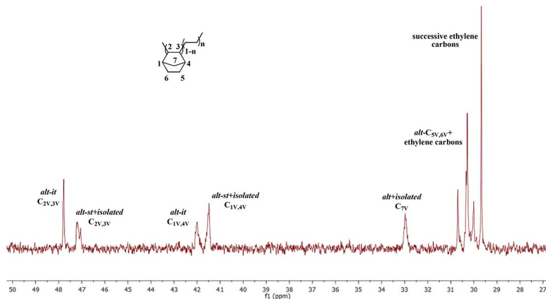
Fig. 5 <sup>13</sup>C NMR spectrum of poly(E)-co-poly(NBE)<sub>VIP</sub> produced by Zr-1/MAO (Table 2, entry 2) (in 1,1,2,2-tetrachloroethane-d<sub>2</sub>).
