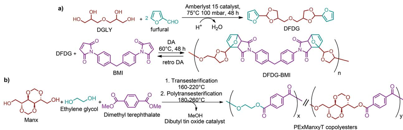
Fig. 30 (a) Thermo-reversible DA polymerization of DFDG and BMI. (b) Production of mannitol based PExManxT copolyesters.
