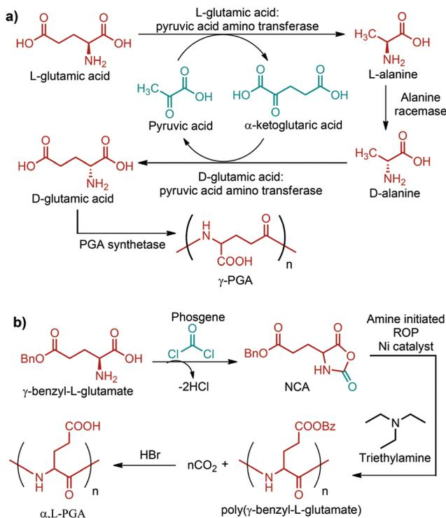
**Fig. 16** (a) Proposed pathway for  $\gamma$ -PGA synthesis from L-glutamic acid in *B. subtilis* IFO 3335 (the pathway starting from glucose to L-glutamic acid was not indicated). (b) Reaction scheme for the synthesis of  $\alpha$ ,L-PGA.
