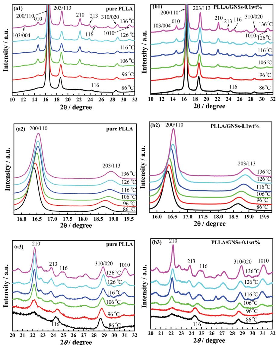
Fig. 1 XRD profiles of pure PLLA and PLLA/GNS composite samples isothermally crystallized at various  $T_c$ s from melt (a1)–(a3) pure PLLA, (b1)–(b3) PLLA/GNS-0.1 wt% composites.
