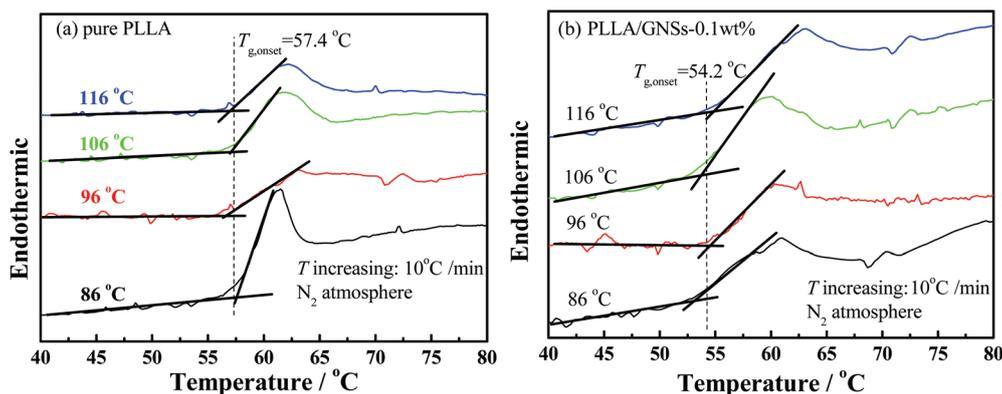
Fig. 7 Determination of glass transition temperatures of PLLA by DSC with a temperature increasing rate of  $10\text{ °C min}^{-1}$  for the samples isothermally crystallized at different  $T_c$ s: (a) pure PLLA, (b) PLLA/GNSs-0.1 wt%.
