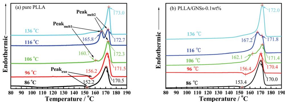
Fig. 12 DSC heating thermographs of pure PLLA and PLLA/GNSs composite samples isothermally crystallized at various  $T_c$ s from the melt: (a) pure PLLA, (b) PLLA/GNSs-0.1 wt%.
