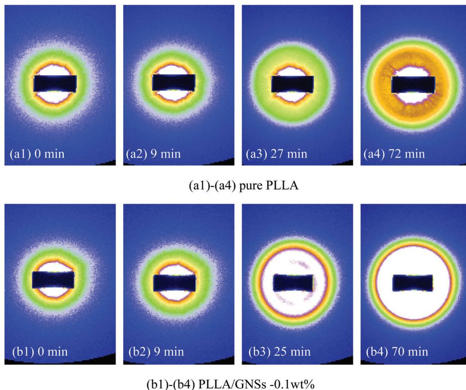
Fig. 9 2D SAXS patterns of pure PLLA and PLLA/GNSs composite samples isothermally crystallized at 145 °C: (a1)–(a4) pure PLLA, (b1)–(b4) PLLA/GNSs-0.1 wt%.
