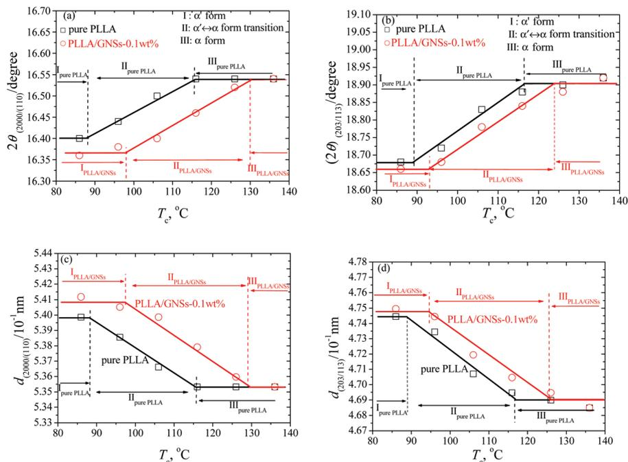
**Fig. 2**  $2\theta$  values from (200)/(110) and (203) diffractions (a and b) and the corresponding  $d$  values calculated from the Bragg equation (c and d) of PLLA and PLLA/GNS composite samples crystallized at various  $T_c$ s from the melt. The lines are plotted to guide the eyes.
