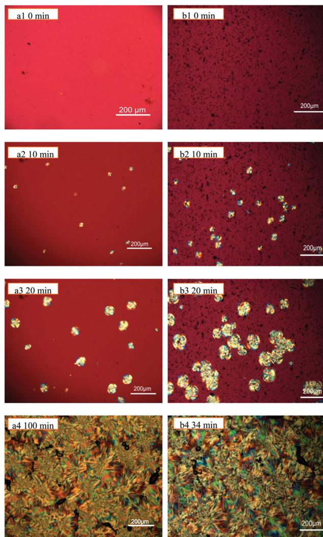
Fig. 3 POM images of PLLA and PLLA/graphene composite samples isothermally crystallized at  $T_c = 140\text{ }^\circ\text{C}$  from melt during their isothermal crystallization process: (a1)–(a4) pure PLLA, (b1)–(b4) PLLA/GNS-0.1 wt% composite.
