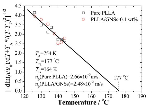
Fig. 8 Analysis of PLLA spherulite growth rate data of pure PLLA and PLLA/GNSs-0.1 wt% composites by fitting with eqn (3) according to the Strobl crystallization theory.
