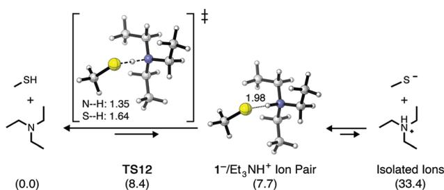
**Scheme 2** Energetics of the acid–base equilibrium between methyl mercaptan (**1**) and triethylamine ( $\text{Et}_3\text{N}$ ) calculated in  $\text{CHCl}_3$ . The relative free energy ( $\Delta G^\circ$  and  $\Delta G^\ddagger$ ,  $\text{kcal mol}^{-1}$ ) of each species or pair of species is given in parentheses. Dashed lines indicate bonds being broken/formed while dotted lines indicate noncovalent interactions. Distances are given in  $\text{\AA}$ .
