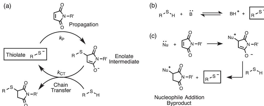
**Scheme 1** (a) Mechanism for the thiolate-catalyzed addition of a thiol to an *N*-substituted maleimide. (b) Formation of a thiolate anion from an acid–base equilibrium reaction. (c) Formation of a thiolate anion following a nucleophile-initiated mechanistic pathway.
