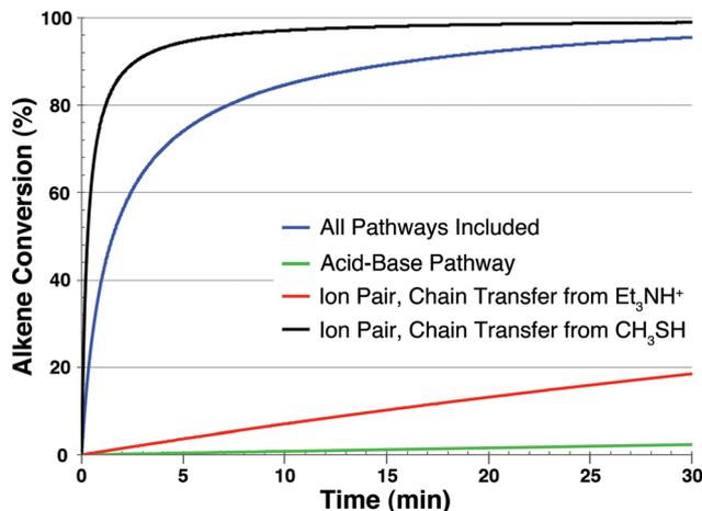
Fig. 5 Results of kinetic modeling of the Et<sub>3</sub>N-mediated addition of methyl mercaptan (**1**) to NMM in CHCl<sub>3</sub>. The blue trace plots alkene conversion when all potential mechanistic pathways discussed in Fig. 2–4 and Scheme 2 are included in the model. The black, red, and green traces selectively exclude specific pathways as a means of evaluating their influence on the overall reaction kinetics.
