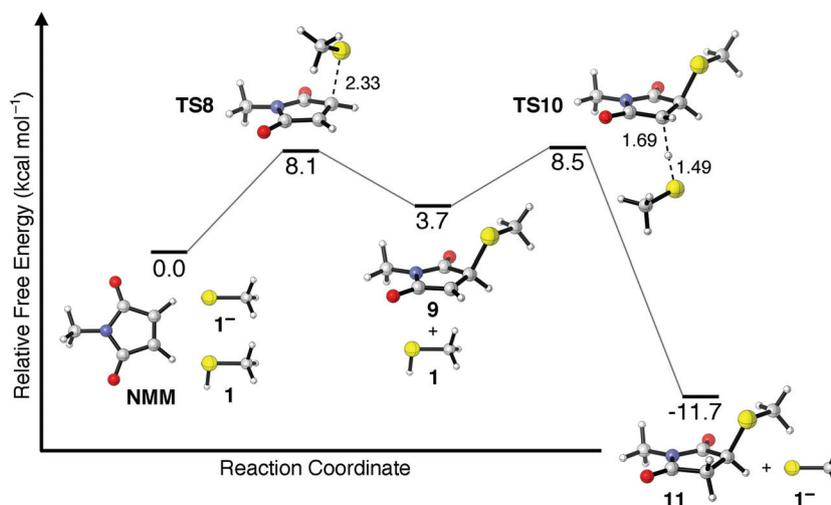
**Fig. 2** Calculated relative free energies of stationary points along the thiolate-catalyzed mechanism of methane thiolate ( $1^-$ ) addition to NMM. Free energies are expressed in  $\text{kcal mol}^{-1}$  and were calculated at 298 K in a solvent model for  $\text{CHCl}_3$ . Distances of bonds breaking or forming in **TS8** and **TS10** are given in angstroms ( $\text{\AA}$ ).
