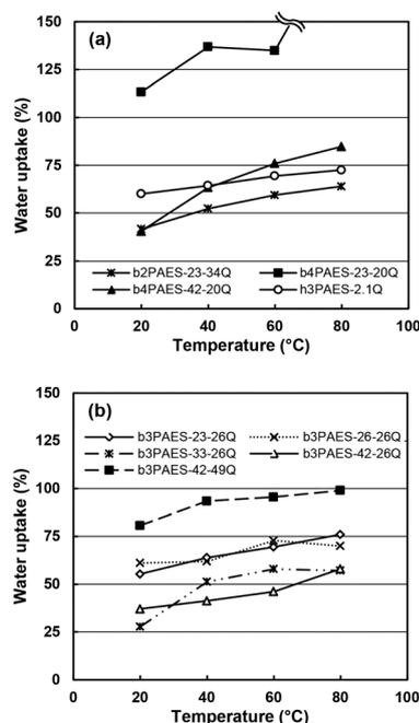
Fig. 6 Water uptake data of the b2PAES-*n*-*m*Q, b4PAES-*n*-*m*Q (a), and the b3PAES-*n*-*m*Q (b) AEMs in the  $\text{Br}^-$  form as a function of temperature under fully hydrated (immersed) conditions. The data is provided in two plots for clarity.
