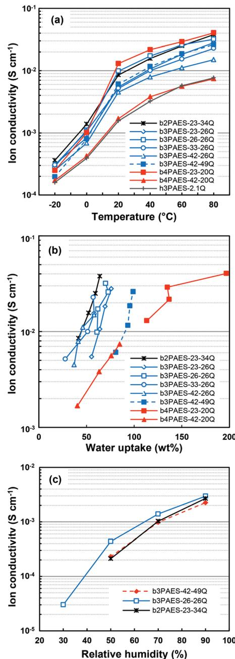
Fig. 7 Br<sup>-</sup> conductivity of the AEMs in the fully hydrated (immersed) state as a function of temperature (a), as a function of water uptake in the temperature range 20–80 °C (b), and as a function of relative humidity at 80 °C (c).
