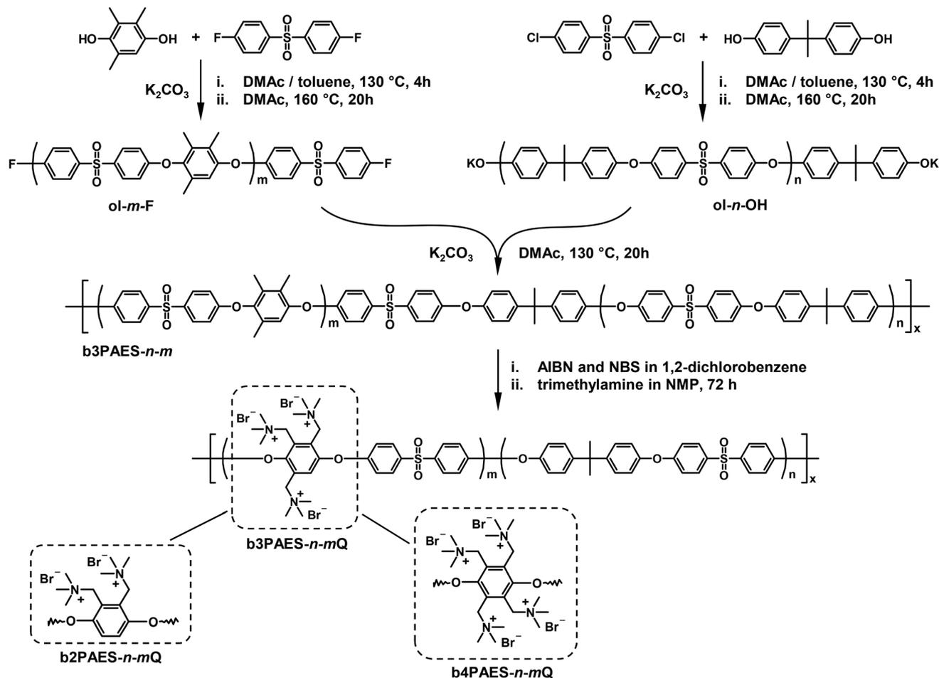
**Scheme 1** Synthetic pathway to the  $b3PAES-n-mQ$  multiblock copolymers by precursor block preparation via polycondensation, block copolymer formation via coupling, and selective benzylic bromination and quaternization. The  $b2PAES-n-mQ$  and  $b4PAES-n-mQ$  multiblock copolymers were prepared using the same method, but by using 2MHQ and 4MHQ, respectively, instead of 3MHQ.
