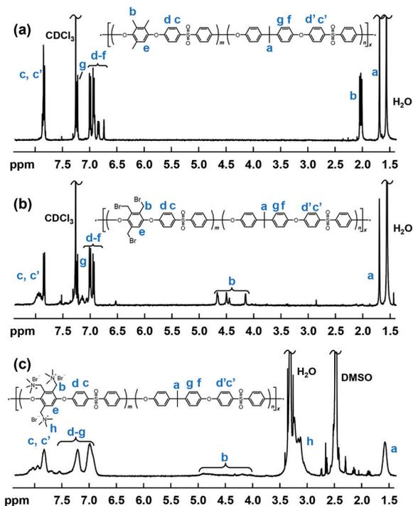
Fig. 2 Representative  $^1\text{H}$  NMR spectra of multiblock copolymers before modification, (a) b3PAES-26-26, after benzylic bromination, (b) b3PAES-26-26Br, and after quaternization, (c) b3PAES-26-26Q.
