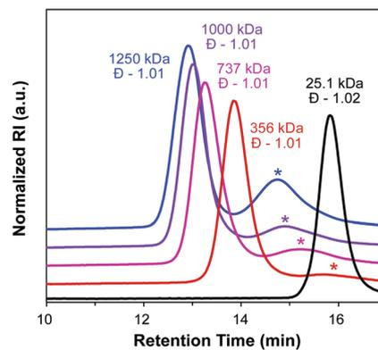
**Fig. 3** RAFT transfer-to mediated by **PCTA1** (black trace), sampled at 19 h (red trace), 42 h (magenta trace), 67 h (purple trace), and 91 h (blue trace). Starred peaks correspond to “dead” polymer. Baselines are shifted for clarity.
