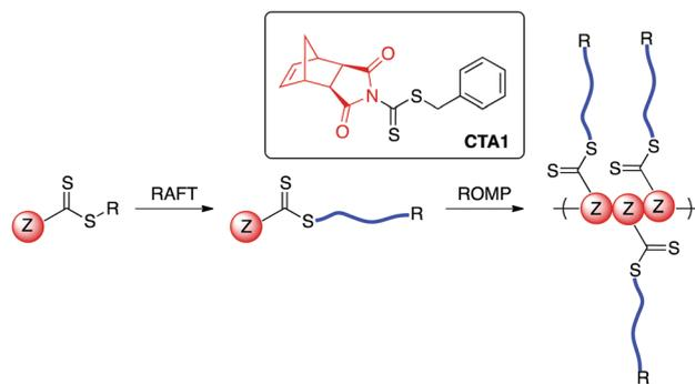
Scheme 1 Proposed CTA structure with directly polymerizable Z-group.
