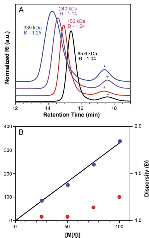
**Fig. 4** Assessment of the livingness of ROMP grafting-through of MM<sub>29</sub>. (A) SEC traces illustrating the increase in MW with increasing [MM<sub>29</sub>]/[G3] ratio (black = [25] : [1], red = [50] : [1], purple = [75] : [1], blue = [100] : [1]). Starred peaks are assigned to residual MMs. Baselines are shifted for clarity. (B) Plot of MW vs. [M]/[I] ratio. The black line represents the theoretical MW for each [MM<sub>29</sub>]/[G3].
