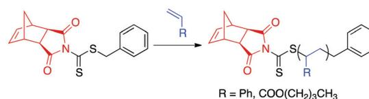
**Scheme 3** CTA1-mediated RAFT polymerization of styrene or *n*BA. <sup>a</sup>Experimental conditions: AIBN, THF, 75 °C for styrene or 60 °C for *n*BA.
