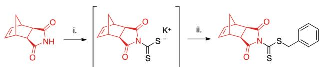
**Scheme 2** One-pot synthesis of CTA1. <sup>a</sup>Experimental conditions: (i) CS<sub>2</sub>, KOH, DMF; (ii) benzyl bromide.
