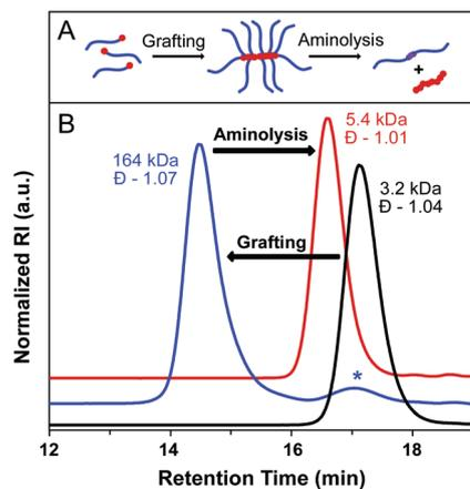
**Fig. 5** (A) Graphical representation of grafting-through and aminolysis. (B) BB synthesis by ROMP grafting-through (blue trace) from  $MM_{29}$  (black trace) and subsequent aminolysis with methylamine (red trace). The starred peak corresponds to residual MM. Baselines are shifted for clarity.
