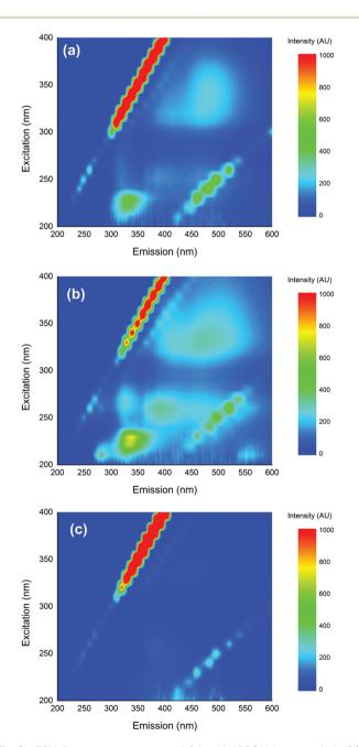
Fig. 2 EEM fluorescence spectra of 0.1 mM 4BPOH in acetonitrile (a), 2-propanol (b) and water (c).
