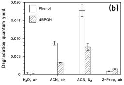
Fig. 6 Degradation rates (a) and degradation quantum yields (b) of phenol and 4BPOH in mixtures (initial concentration 0.1 mM for both compounds), upon UVB irradiation in different solvents (water, acetonitrile, and 2-propanol) and different conditions (air or nitrogen atmosphere). The error bars represent  $\pm \sigma$ . The rates and quantum yields in water were negligible, and only the related uncertainty (detection limit) is reported. ACN = acetonitrile.
