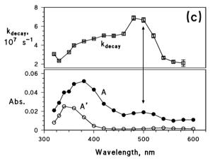
Fig. 5 (a) Upper plot: first-order decay constant ( $k_{\rm decay}$ ) of the laser trace as a function of wavelength, upon irradiation (355 nm, 94 mJ per pulse) of 0.1 mM benzophenone in 1:12-propanol: acetonitrile. Lower plot: maximum absorbance of the laser trace under the same conditions. (b) Laser trace (350 nm) upon irradiation of 0.1 mM 4BPOH in 1:12-propanol: acetonitrile (355 nm, 94 mJ per pulse). The absorbance values A and A' and the time interval used to determine  $k_{
