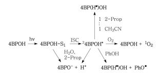
Scheme 1 Hypothesised processes involving the transient species formed upon irradiation of 4BPOH. 2-Prop: 2-propanol; PhOH: phenol; PhO: phenoxyl; ISC: inter-system crossing.
