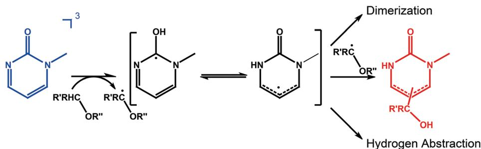
**Fig. 5** Scheme summarizing HA by  $^3\text{1MP}^*$ . 1MP in the triplet state abstracts a hydrogen atom from the quencher bearing a  $-\text{CRH}-\text{O}-$  chemical motif. The so formed radical can tautomerize forming a NH group. Recombination with the quencher radical terminates the reaction chain. For high concentrations also dimerization could occur.
