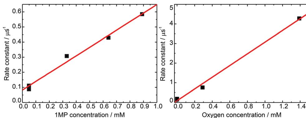
**Fig. 3** Rate constants for the triplet decay of 1MP. Rate constants are determined from exponential fits to time traces at a detection wavelength of 430 nm (squares). A linear fit to that data (lines) yields the corresponding quenching rate constants. (Left) Concentration dependence of the triplet decay in de-oxygenated solutions. (Right) Quenching by molecular oxygen at a 1MP concentration of 75  $\mu$ M.
