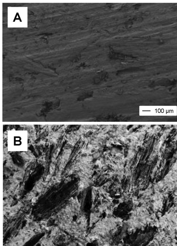
**Fig. 3** Scanning electron micrograph of a WPC (white oak (60%)/HDPE (40%) control sample (A) and after exposure to *Gloeophyllum trabeum* (Brown rot fungi) for 12 weeks (B). Reproduced with permission from Fabiyi *et al.*<sup>39</sup>
