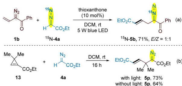
Scheme 6 (a) The cross-coupling of 1b with ^{15}\text{N} - 4a ; (b) the reaction of stable cyclopropane 13 with ethyl diazoacetate 4a .
