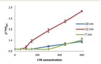
**Fig. 9** Plot of the ratio of the absorbance intensity at 620 nm both with and without LTB vs. LTB concentration (nM) for Gal-gAuNPs of different sizes. Each point is the average of three measurements with the error bars representing the standard error.
