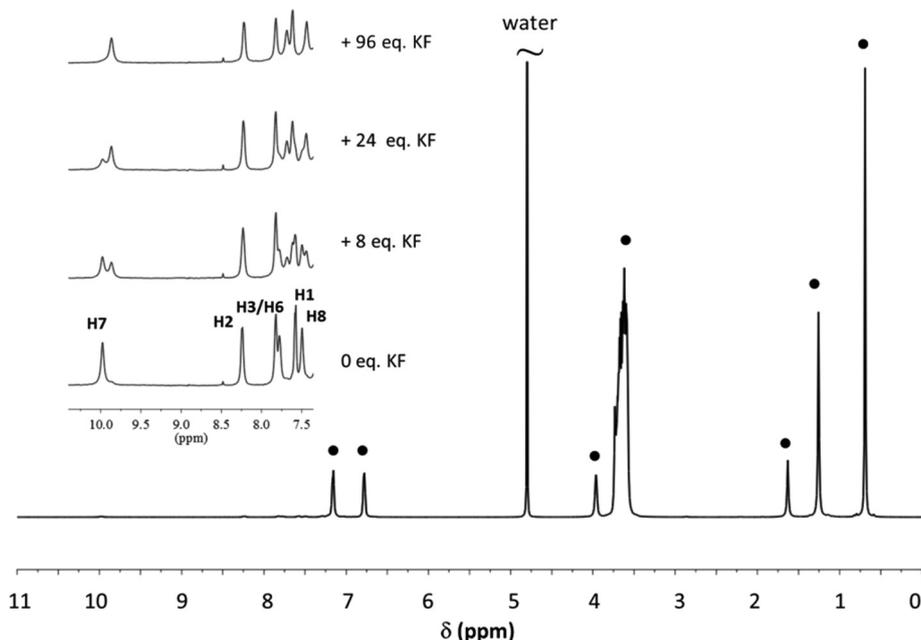
**Fig. 3**  $^1\text{H}$  NMR spectrum of a 1.5 mM solution of Receptor 2 in 50 mM Triton X-100. Receptor signals are amplified and shown for different additions of KF. (●) Surfactant signals. The assignment of the receptor signals was made by comparison with the spectrum of the receptor in CTAX micelles. For proton labelling see Fig. 1.
