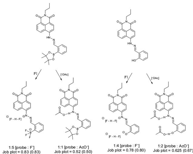
**Scheme 1** Proposed binding modes for probes **1** and **2** with fluoride and acetate anion in MeCN. Stoichiometry of binding and Job plot analysis: observed value and (theoretical) value.
