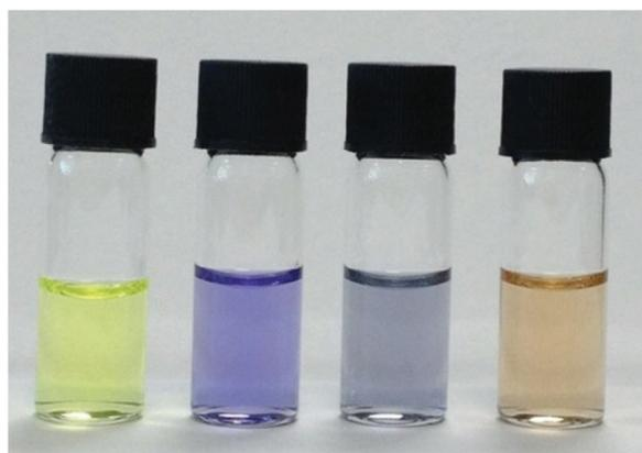
Fig. 4 Colour changes of probe 1 after treatment with different anions. Samples show, from left to right: 12  $\mu\text{M}$  probe 1, 13 equiv. of each anions or the anions  $\text{F}^-$ ,  $\text{OAc}^-$ ,  $\text{H}_2\text{PO}_4^-$  respectively.
