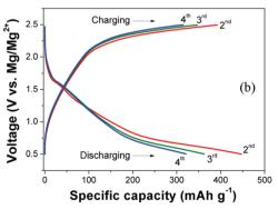
Fig. 8 (a) Initial and (b)  $2^{nd}$ ,  $3^{rd}$  and  $4^{th}$  charge-discharge curves of the S-rGO nanocomposite at a current density of 20 mA  $g^{-1}$  in the voltage range of 0.5–2.5 V vs. Mg/Mg<sup>2+</sup>.
