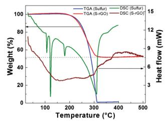
Fig. 4 TGA-DSC analysis of sulfur and S-rGO nanocomposites under 20 ml min<sup>-1</sup> helium flow and 10 °C min<sup>-1</sup> heating rate.
