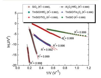
Fig. 5 Fowler–Nordheim plots in the forward biasing condition show excellent linear behavior in the tunnel barriers, strong evidence of F-N tunneling.
