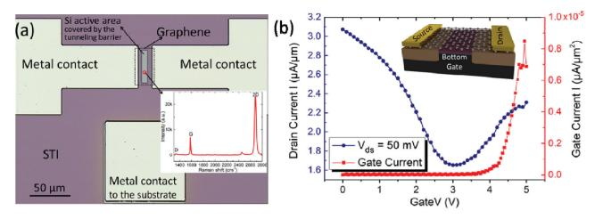
Fig. 2 (a) Top-view micrograph of a fabricated device with the graphene Raman fingerprint shown as an inset. The Raman spectrum confirms the presence of the single layer graphene with a very small in-plane crystal defect related peak (D peak). (b) Transfer characteristics (blue circles) and gate leakage current (red squares) of a GFET with a 5 nm Al<sub>2</sub>O<sub>3</sub>/HfO<sub>2</sub> gate dielectric stack. The inset shows the schematic of the back gated GFET.
