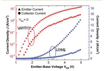
Fig. 8 Transfer characteristics of a GBT with the TmSiO/TiO2 emitter tunnel barrier and a 60 nm deposited Si as the BCI. The left and righthand axes (red and blue) show the current on logarithmic and linear scales, respectively. While the triangles show the emitter current and the circles display the collector current. The collector current has dramatically improved in comparison with previously reported GBTs with the on-state current densities in the order of 10 µA cm<sup>-2</sup> (ref. 9).
