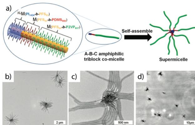
**Fig. 18** Hierarchical, crystallization-driven growth of MCNs. (a) Schematic of the sequential block crystallization to ABC block ter-micelles. (b, c) TEMs of the supermicelles obtained from higher level self-assembly using ABC block ter-micelles as building blocks. (d) Optical microscopy image of the micron-sized supermicelles. Reprinted from ref. 303 with permission from American Association for the Advancement of Sciences.
