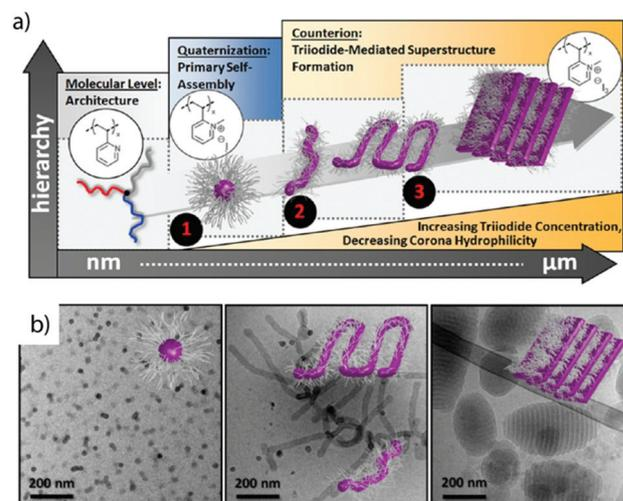
**Fig. 16** Counterion-mediated structuring of  $\mu$ -(BVqT)<sup>+/I<sup>–</sup></sup> miktoarm star terpolymers in water. (a) Hierarchical self-assembly mechanism and morphological evolution with iodine self. (b) Spherical micelles, worm-like micelles and axially stacked lamellae in ellipsoidal MCNs. Reprinted from ref. 299 with permission from American Chemical Society.
