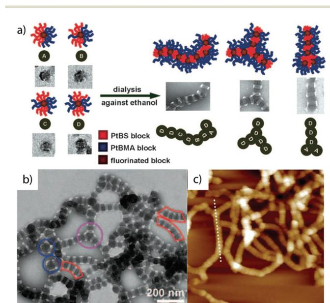
**Fig. 19** Hierarchical self-assembly of patchy micelles. (a) Step-wise self-assembly involving first the collapse of P<sub>f</sub>B middle block of PtS-*b*-P<sub>f</sub>B-*b*-PtBMA followed by stacking of patchy micelles to linear undulated MCNs. (b, c) TEM image illustrating the internal segmentation of cylindrical micelles into P<sub>f</sub>B (bright) and PtS (dark) compartments and AFM showing topography of the undulated cylinders. Reprinted from ref. 305 with permission from Wiley-VCH.
