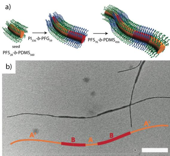
**Fig. 5** Crystallization-driven self-assembly of cylindrical micelles. (a) Schematic of growth mechanism to alternating core and corona compartments. (b) TEM image of pentablock co-micelle with bifunctional crystalline nucleus (orange) of PFS-*b*-PDMS, extended with PFG-*b*-PI (red) and again with PFS-*b*-PDMS. Reprinted from ref. 146 with permission from Nature Publishing Group.
