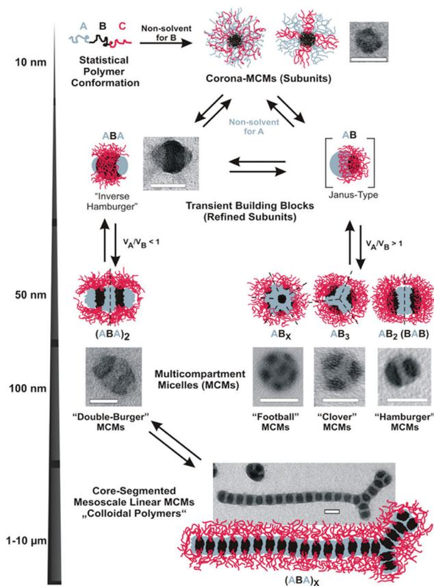
**Fig. 20** Schematic of MCN formation using non-solvent sequences for linear triblock terpolymers. The series of TEM images shows the underlying self-assembly mechanism involving dispersion of SBM triblock terpolymer in a non-solvent for PB to patchy micelles and subsequent collapse of PS patches into spherical or cylindrical MCNs depending on  $V_{PS}/V_{PB}$ . Reprinted from ref. 84 with permission Nature Publishing Group.
