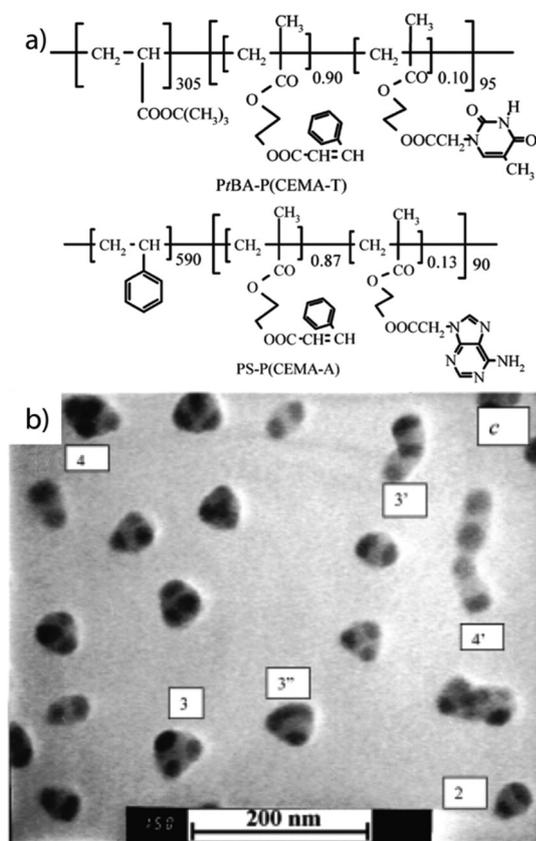
**Fig. 14** MCNs of chemically stitched triblock terpolymer. (a) Diblock copolymers modified with complementary DNA base-pair derivatives. (b) MCNs with a PS core, two to four compartments of chemically stitched P(CEMA-A/T) stabilized by a PtBA corona. Reprinted from ref. 281 with permission from American Chemical Society.
