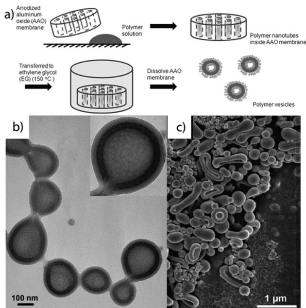
**Fig. 12** Rehydration of bulk films in AAO channels. (a) Processing steps comprise: AAO template-assisted shearing of PI-*b*-PS-*b*-P2VP, annealing in selective solvents at elevated temperatures followed by rehydration and release of vesicles. (b, c) TEM and SEM characterization of vesicles with mesh-like membrane morphology. Reprinted from ref. 269 with permission from American Chemical Society.
