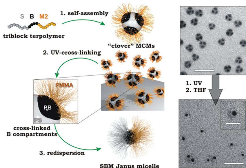
**Fig. 23** Solution-based approach to produce SBM Janus nanoparticles. Self-assembly of SBM triblock terpolymer into MCNs, crosslinking of PB compartments and re-dispersion in good solvent for all blocks releases Janus nanoparticles. TEM images show MCNs before cross-linking and individual Janus nanoparticles after re-dispersion. Reprinted from ref. 325 with permission from American Chemical Society.
