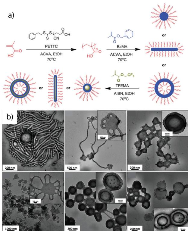
**Fig. 10** Polymerization-induced self-assembly. (a) Schematic of sequential RAFT polymerization to poly(methacrylic acid) in water followed by emulsion polymerization of poly(benzyl methacrylate) and poly(2,2,2-trifluoroethyl methacrylate). (b) Morphologies after PISA of the three blocks and structural evolution from spheres/cylinders to cylinders and vesicles. Reprinted from ref. 238 with permission from Royal Society of Chemistry.
