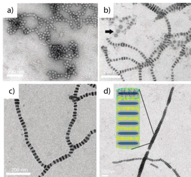
**Fig. 15** Linear superstructures based on step-wise self-assembly. (a) Self-assembled disc-like PS-*b*-PMA-*b*-PAA micelles and (b) stacking into (c) extended segmented cylinders directed by solvent mixtures and additives. (d) The polyionic complex allows for selective storage of cargo, here gold particles. Reprinted from ref. 284 with permission from American Association for the Advancement of Sciences.
