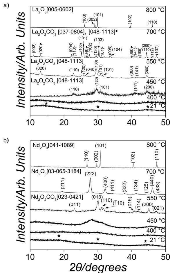
**Fig. 1** Selected powder X-ray diffraction patterns recorded from the lanthanum (a) and neodymium (b) solid precursor phases (bottom patterns in both cases) and their crystallization products when dry-heated from 25 °C to 1000 °C. The asterisks in the bottom patterns indicate the position of the humps in the amorphous precursors.
