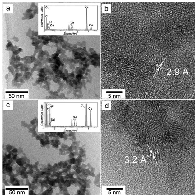
**Fig. 2** TEM images of the pristine amorphous lanthanum (a) and neodymium (c) carbonate precursor phases and the crystalline transformation products produced by irradiation with the high energy electron beam of the TEM for a few seconds (b and d respectively). The insets show the respective EDX spectra with the Cu peaks coming from the Cu support grid. Standardless quantification from these spectra gave a La : O and Nd : O atomic ratio of 2 : 8.
