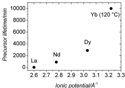
Fig. 9 Plot showing the proportionality between the stability of the La, Nd, Dy and Yb amorphous carbonate precursors and the ionic potential of the REE<sup>3+</sup> involved in the precursor.
