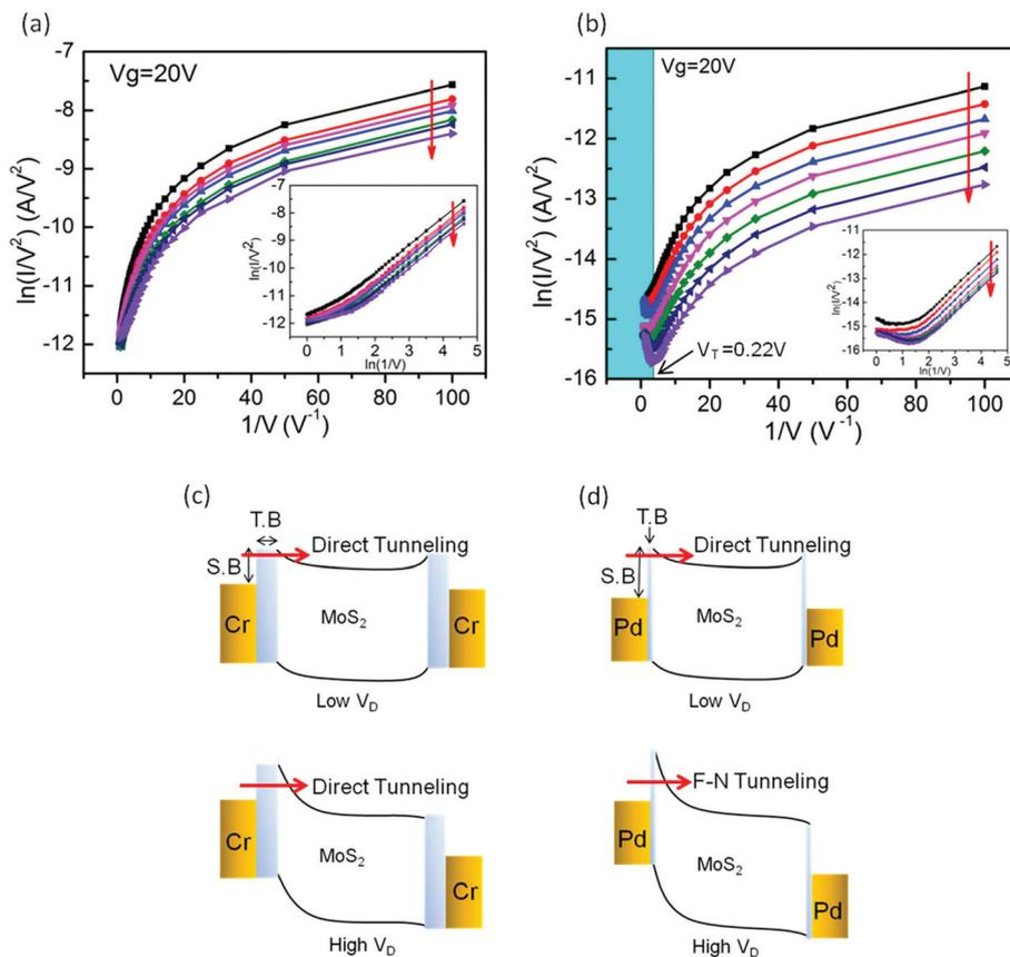
**Fig. 2**  $\ln(I/V^2)$  plotted vs. the inverse of the drain bias ( $1/V$ ): (a) for the Cr contact and (b) for the Pd contact. Insets show the same plot with logarithmic abscissa. The arrows denote a decrease in the temperature from room temperature down to 123 K. (c) and (d) The band diagrams of (a) and (b), where SB and TB denote a Schottky barrier and a tunnel barrier, respectively. Note that  $0 \leq V_D \leq 1$ .
