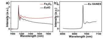
Fig. 3 (a) Fe K-edge XAS spectra of EulO nanocubes and Fe $_3O_4$  nanoparticles, (b) Eu L $_{III}$ -edge XAS spectrum of EulO nanocubes. The absorption peaks are attributed to the  $2p_{3/2}/5d$  electron transition for the trivalent Eu L $_{III}$ -edges.
