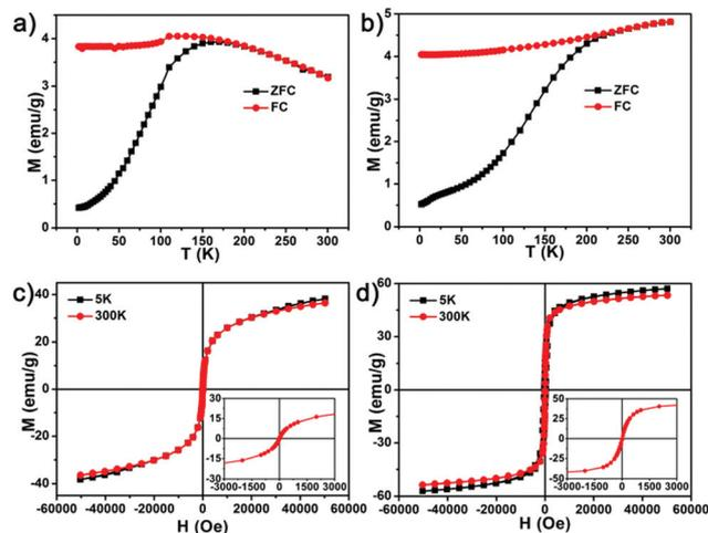
**Fig. 4** Magnetic properties. Temperature dependent magnetization curves under ZFC/FC conditions of (a) EuIO nanocubes and (b) magnetite nanoparticles under an applied magnetic field of 50 Oe. Field-dependent magnetization curves ( $M$ - $H$ ) of (c) EuIO nanocubes and (d) magnetite nanoparticles at 300 K and 5 K (insets: magnification of  $M$ - $H$  curves from  $-3000$  to  $3000$  Oe at 300 K).
