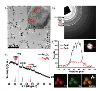
Fig. 2 Characterization of EulO nanocubes. (a) Representative TEM image of 14 nm sized monodispersed EulO nanocubes (inset: HRTEM image). (b) XRD and (c) SEAD patterns of EulO nanocubes. (d) EDX line profiles across a EulO nanocube (inset: a scanning TEM image with high angle annular dark field, STEM-HAADF image). (e) EDX mapping images of EulO nanocubes (inset: STEM-HAADF image of relative EulO nanocubes)
