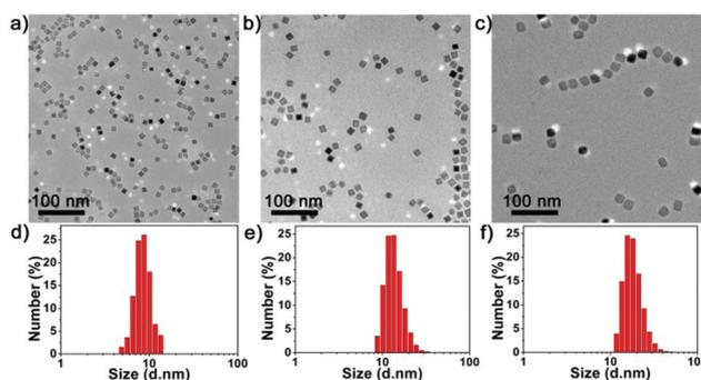
**Fig. 1** TEM images (a–c) and the related DLS analysis profiles (d–f) of monodispersed EuIO nanocubes with different sizes: (a, d)  $10.0 \pm 1.7$  nm, (b, e)  $14.0 \pm 1.9$  nm, and (c, f)  $20.1 \pm 2.4$  nm.
