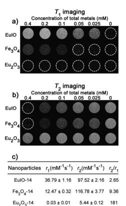
Fig. 5 MRI contrast enhancement performance of EulO nanocubes compared to Fe<sub>3</sub>O<sub>4</sub> and Eu<sub>2</sub>O<sub>3</sub> nanoparticles with similar sizes of about 14 nm. (a)  $T_1$ -weighted and (b)  $T_2$ -weighted phantom imaging of 14 nm sized EuIO nanocubes, magnetite and Eu<sub>2</sub>O<sub>3</sub> nanoparticles on a 0.5 T MRI scanner. (c) The  $r_1$  and  $r_2$  values of EuIO nanocubes, Fe<sub>3</sub>O<sub>4</sub> and Eu<sub>2</sub>O<sub>3</sub> nanoparticles.
