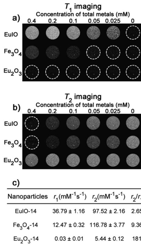
Fig. 5 MRI contrast enhancement performance of EuIO nanocubes compared to  $\text{Fe}_3\text{O}_4$  and  $\text{Eu}_2\text{O}_3$  nanoparticles with similar sizes of about 14 nm. (a)  $T_1$ -weighted and (b)  $T_2$ -weighted phantom imaging of 14 nm sized EuIO nanocubes, magnetite and  $\text{Eu}_2\text{O}_3$  nanoparticles on a 0.5 T MRI scanner. (c) The  $r_1$  and  $r_2$  values of EuIO nanocubes,  $\text{Fe}_3\text{O}_4$  and  $\text{Eu}_2\text{O}_3$  nanoparticles.
