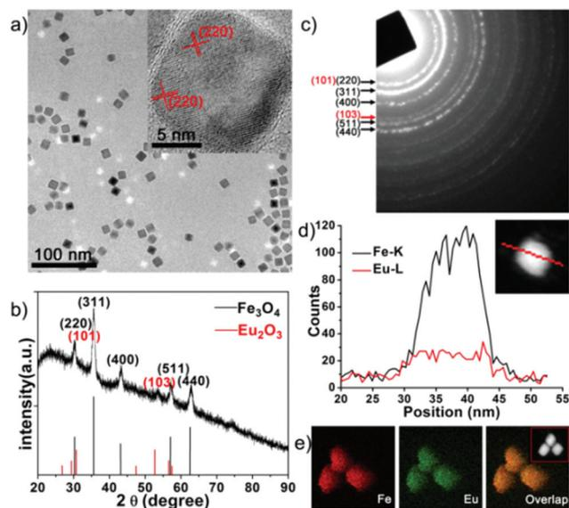
**Fig. 2** Characterization of EuIO nanocubes. (a) Representative TEM image of 14 nm sized monodispersed EuIO nanocubes (inset: HRTEM image). (b) XRD and (c) SAED patterns of EuIO nanocubes. (d) EDX line profiles across a EuIO nanocube (inset: a scanning TEM image with high angle annular dark field, STEM-HAADF image). (e) EDX mapping images of EuIO nanocubes (inset: STEM-HAADF image of relative EuIO nanocubes).
