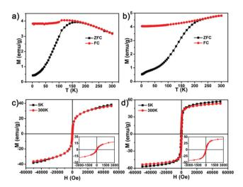
Fig. 4 Magnetic properties. Temperature dependent magnetization curves under ZFC/FC conditions of (a) EulO nanocubes and (b) magnetite nanoparticles under an applied magnetic field of 50 Oe. Field-dependent magnetization curves (M-H) of (c) EulO nanocubes and (d) magnetite nanoparticles at 300 K and 5 K (insets: magnification of M-H curves from -3000 to 3000 Oe at 300 K).
