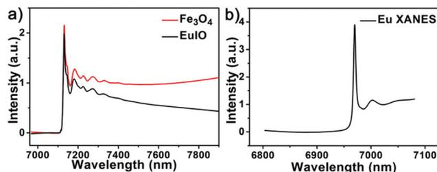
**Fig. 3** (a) Fe K-edge XAS spectra of EuIO nanocubes and  $\text{Fe}_3\text{O}_4$  nanoparticles, (b) Eu  $L_{\text{III}}$ -edge XAS spectrum of EuIO nanocubes. The absorption peaks are attributed to the  $2p_{3/2}/5d$  electron transition for the trivalent Eu  $L_{\text{III}}$ -edges.
