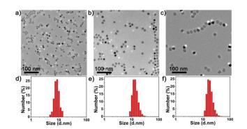
Fig. 1 TEM images (a-c) and the related DLS analysis profiles (d-f) of monodispersed EulO nanocubes with different sizes: (a, d) 10.0 + 1.7 nm, (b, e)  $14.0 \pm 1.9$  nm, and (c, f)  $20.1 \pm 2.4$  nm.
