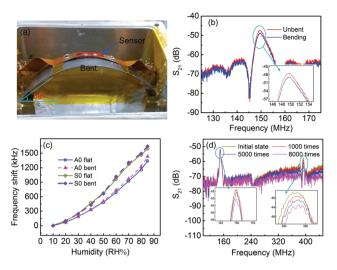
Fig. 7 Photograph of the sensor at a bent state (a); comparison of transmission spectra (b), frequency shifts of a flexible humidity sensor ( $\lambda$  = 12  $\mu$ m, D3) unbent and bent at an angle of 36°(c), and (d) the dependence of the transmission properties of the sensor as a function of bending cycles.
