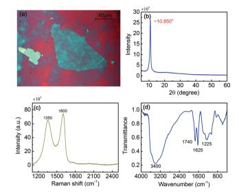
Fig. 3 A microscopy image of the graphene oxide microflakes on the SiO<sub>2</sub>/Si substrate (a); an X-ray diffraction curve (b); Raman spectrum recorded with  $\lambda_{exc}$  = 532 nm (c), and FTIR spectrum (d) of the GO film.
