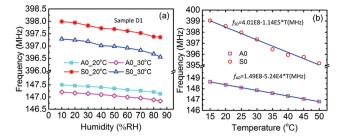
Fig. 6 The resonant frequency of D1 as a function of humidity at 20  $^{\circ}$ C and 30  $^{\circ}$ C (a) and as a function of temperature at 30%RH (b). The temperature coefficient of frequency for both the wave modes has an excellent linearity with the correlation coefficient of 0.9996 for A0 and 0.9832 for S0.
