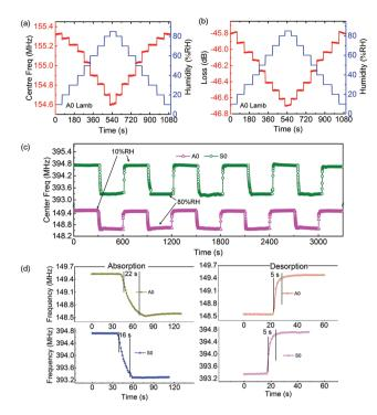
Fig. 5 Detailed responses of the resonant frequency shift (a) and insertion loss (b) of the A0 mode, sample D3 to humidity change; the repeatability of the frequency of the AO and SO (c) modes of sample D3 when the humidity was repeatedly changed from 10%RH to 80%RH. (d) Detailed frequency response curves, showing the response and recovery times of the sensor (D3).
