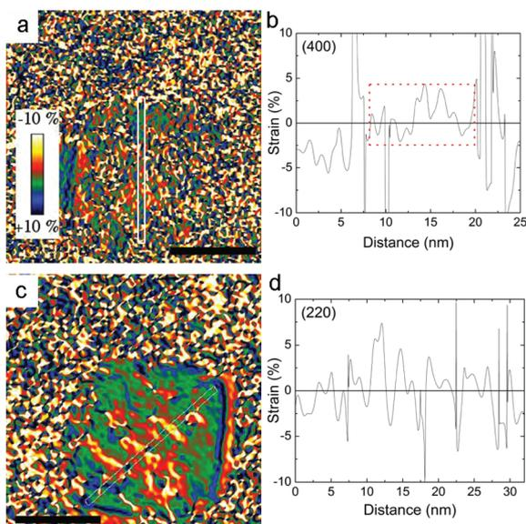
**Fig. 3** Deformation maps obtained through the GPA of the (a)  $g_{200}(\text{wüstite})/g_{400}(\text{spinel})$  and (c)  $g_{220}(\text{spinel})$  reflections for the CS\_45 nanoparticles (scale bar = 25 nm). (b) and (d) show the corresponding integrated line profiles. The boxed region in the graph indicates the probable position of the  $\text{Fe}_3\text{O}_4$  core.
