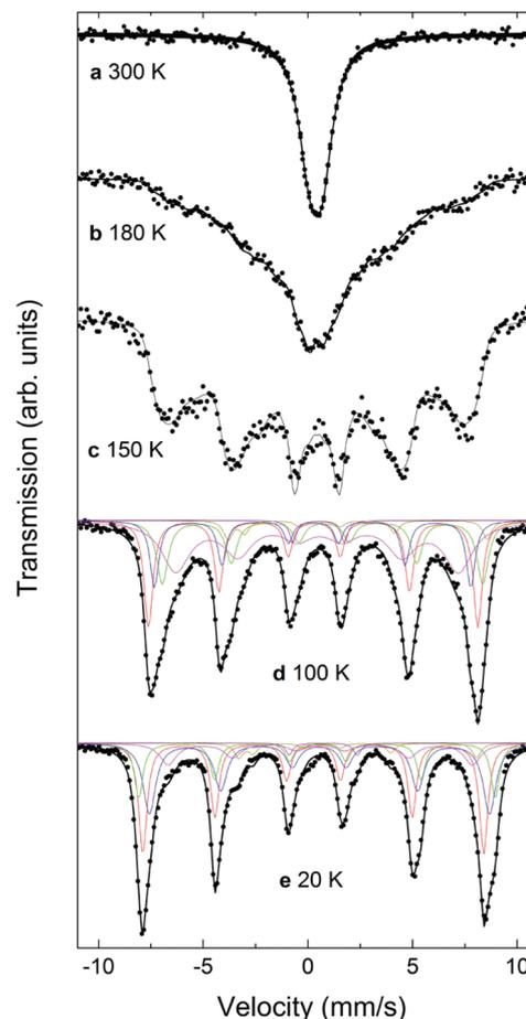
**Fig. 7** Mössbauer spectra for the CS\_9 particles at (a) 300 K, (b) 180 K, (c) 150 K, (d) 100 K, and (e) 20 K. Note that the fact that a fit with only two discrete sextets for  $Fe_3O_4$  did not lead to satisfactory results can be interpreted as a clear evidence of the charge ordering in the CS\_9 particles at these temperatures, although no Verwey transition can be identified.
