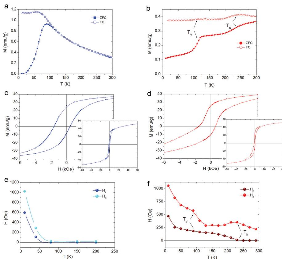
**Fig. 5** Temperature dependence of the field cooled (FC) and zero field cooled (ZFC) magnetizations for (a) CS\_9 and (b) CS\_45 particles. Enlarged view at a low field of the hysteresis loops at 10 K for (c) CS\_9 and (d) CS\_45 nanoparticles. The insets show the hysteresis loops in the full field range. Temperature dependence of the coercivity,  $H_{\text{C}}$ , and the loop shift,  $H_{\text{E}}$ , for (e) CS\_9 and (f) CS\_45 nanoparticles. The lines are guides to the eye.
