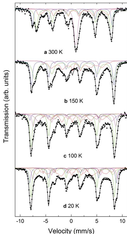
**Fig. 8** Mössbauer spectra for the CS\_45 particles at (a) 300 K, (b) 150 K, (c) 100 K, and (d) 20 K. The characteristics of the two resolved sextets correspond to  $\text{Fe}^{3+}$  in the tetrahedral (A) sites (the outermost sextet, 20%), and to  $\text{Fe}^{2+}$  and  $\text{Fe}^{3+}$  in the octahedral (B) sites (36%).
