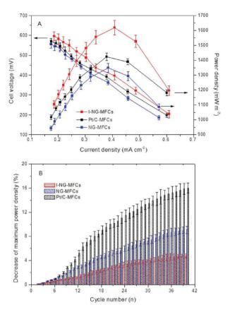
Fig. 5 (A) Power densities and cell voltages of mesoporous graphitic C<sub>3</sub>N<sub>4</sub>-NG MFCs, regular NG-MFCs and Pt/C-MFCs. (B) Reduction of maximum power density with cycle number at an external resistance of 1000  $\Omega$ . Reproduction with permission from ref. 67.
