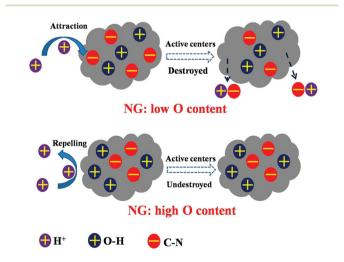
Fig. 6 NG is protected by O-H groups from the attack of protons. Reproduction with permission from ref. 56.
