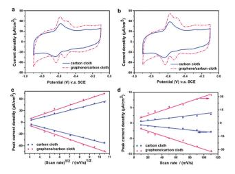
Fig. 4 (A) Cyclic voltammograms of MFC in glucose-free medium and (B) in 0.5% glucose medium at a scan rate of 30 mV s $^{-1}$ . (C) Peak current of Peak 1 (-0.6 V vs. SCE) is plotted *versus* the square root of scan rate. (D) Peak current of Peak 2 (-0.5 V vs. SCE) is plotted *versus* scan rate. Reproduction with permission from ref. 45.
