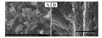
**Fig. 3** (A) Morphology of crumpled r-GO particles. (B) SEM images of the attachment of bacterial cells on the graphene/PANI anodes. Reproduction with permission from ref. 42, 43.
