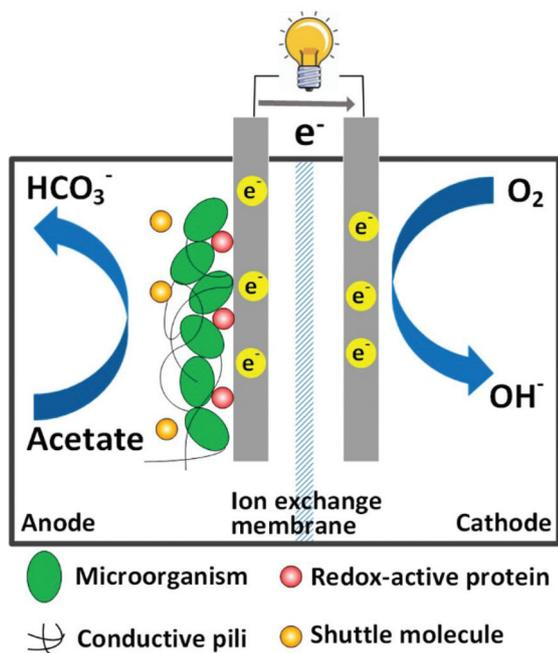
Fig. 1 Schematic of a typical two-chamber MFC.
