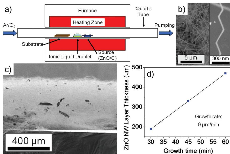
**Fig. 1** (a) Schematic diagram of the one-zone (1 in. quartz tube) thermal CVD setup to grow ZnO nanowires by an IL assisted approach. The IL droplet is placed in the upstream direction from the ZnO/C powder source. (b) SEM micrograph of the *a*-axis VLS ZnO nanowires. The inset shows the kinking from the *a*-axis nanowire growth. (c) Cross-sectioned SEM micrograph of IL ZnO nanowires. (d) Plot of ZnO nanowire layer thickness versus the growth time to determine the growth rate.
