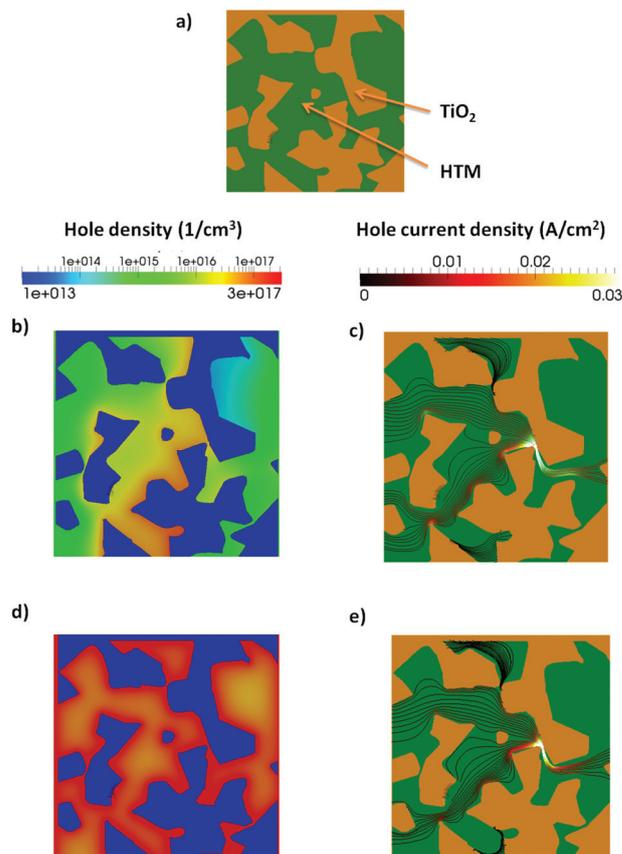
Fig. 7 (a) The RM region with the TiO<sub>2</sub> (orange) and the Spiro-OMeTAD (green). (b) Hole density and (c) hole current density at  $J_{sc}$  for the case without trapped electrons at the TiO<sub>2</sub>/HTM interface. (d) and (e) are the same as (b) and (c) but with trapped electrons at the interface.
