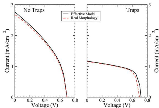
**Fig. 2** (Left)  $J$ - $V$  characteristics without trap states at the interface with and without real morphology in the middle of the cell. (Right) the same as in the left but adding the trap states at the interface.
