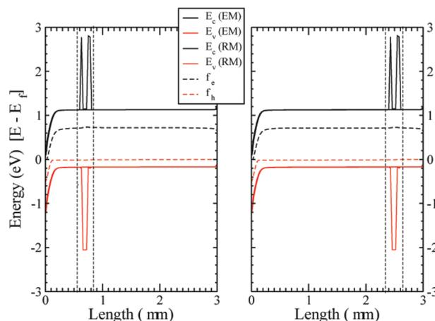
**Fig. 3** Conduction and valence bands (LUMO and HOMO level for the HTM)  $E_c$  and  $E_v$  and electrochemical potentials for electrons  $\phi_e$  and holes  $\phi_h$  at  $J_{\text{sc}}$  for different positions of the RM region. Close to the anode (left) and close to the cathode (right). The band bending is compared to calculations using the effective approximation (EM) only. The RM region is delimited by the vertical broken lines.
