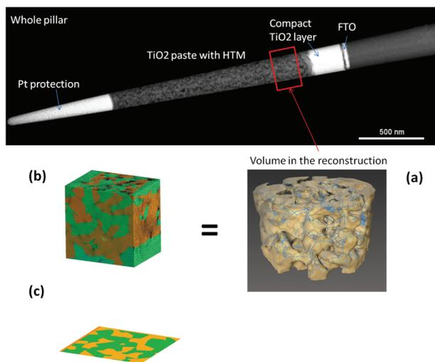
**Fig. 4** (Top) High angle annular dark field (HAADF) STEM image. (a) Reconstruction of the  $\text{TiO}_2$  morphology in a portion of the active layer. (b) Meshing of a cube extracted from the measurement of the  $\text{TiO}_2$ , reconstructing the HTM phase. (c) 2D slice of the 3D morphology.
