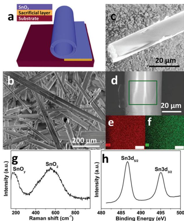
**Fig. 1** Fabrication and characterizations of the as-obtained SnO<sub>2</sub> nanomembranes: (a) fabrication scheme, (b) overall SEM image, (c–d) a single rolled-up nanomembrane, (e) Sn and (f) O element mapping images (scale bar: 6 μm) of the selected area in (d), (g) Raman and (h) Sn 3d XPS spectrum.
