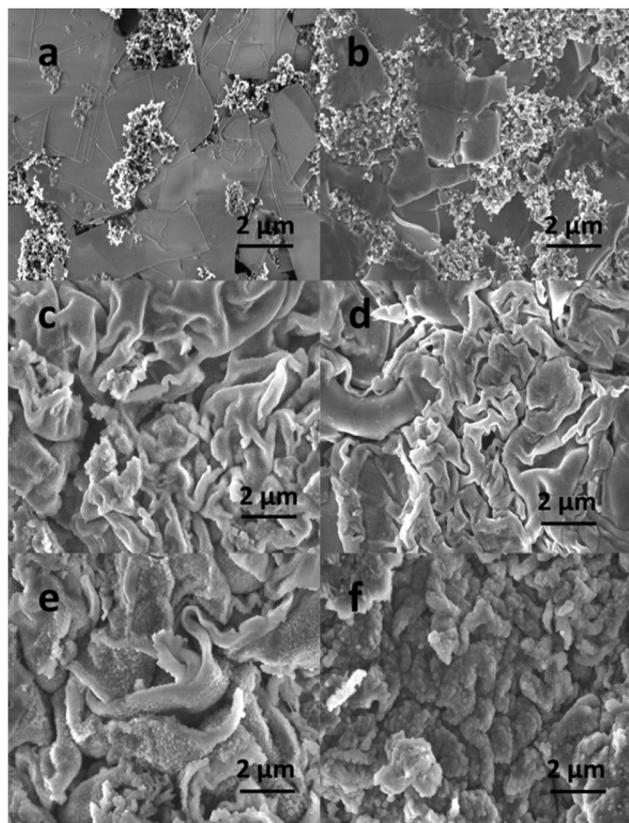
Fig. 5 SEM images of the SnO<sub>2</sub> nanomembrane electrodes: (a) before cycling, (b) after the 1st cycle, (c) and (d) after 100 cycles ((d): without carbon black), (e) after 300 cycles and (f) 900 cycles at 1600 mA g<sup>-1</sup>.
