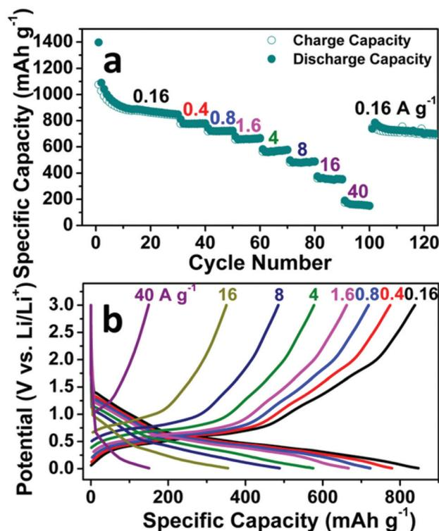
Fig. 4 Rate capability of the SnO<sub>2</sub> nanomembrane electrode: (a) Rate cycling performance, (b) Representative discharge/charge voltage curves at various current rates.
