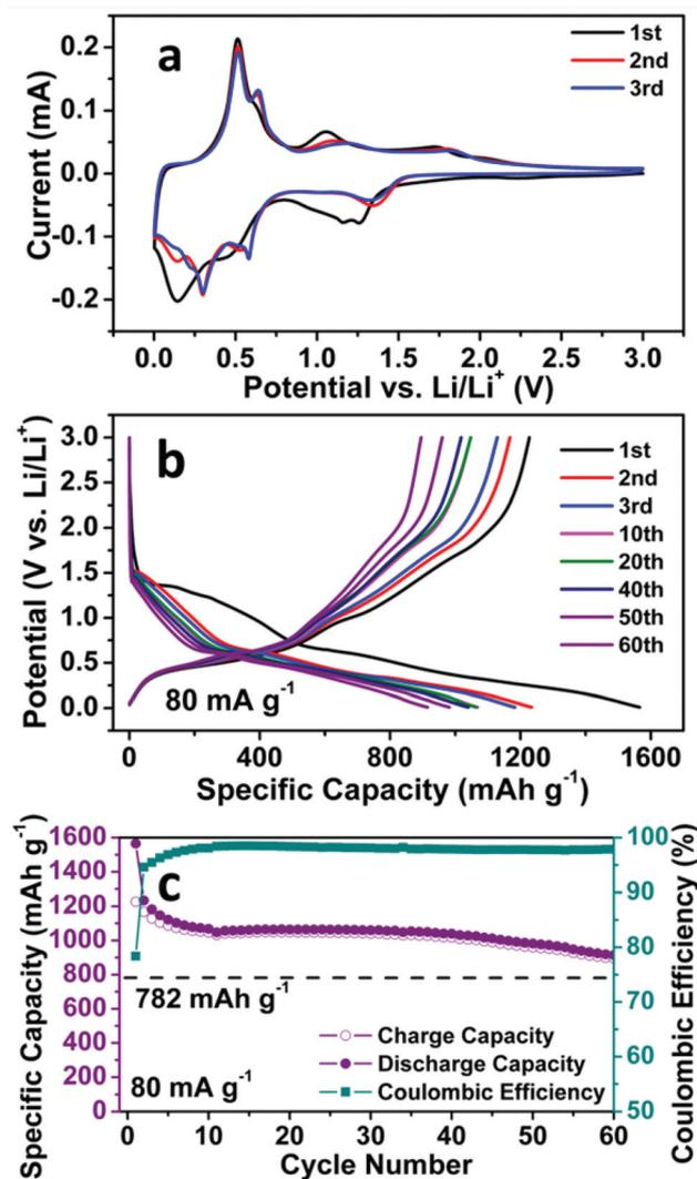
Fig. 2 (a) CV curves, (b) Representative discharge/charge voltage curves at 80 mA g<sup>-1</sup>, and (c) Cycling performance at 80 mA g<sup>-1</sup> of the SnO<sub>2</sub> nanomembrane electrodes.
