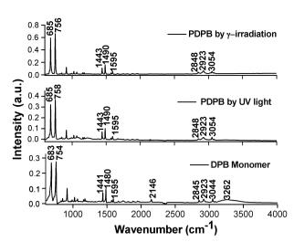
**Fig. 2** ATR-FTIR spectra of pure DPB monomer (bottom spectrum), and PDPB nanostructures synthesized either by UV light irradiation (middle spectrum), or by gamma irradiation (top spectrum) with  $\phi = 2.21$ ,  $C_{\rm s} = 0.3$  mol L $^{-1}$ .
