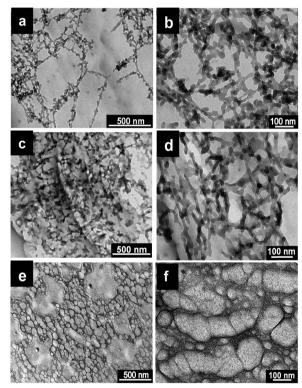
**Fig. 4** Transmission electron micrographs of PDPB nanostructures prepared by UV-irradiation in mesophases with (a and b)  $\phi$  =2.21 and  $C_{\rm s}$  = 0.3 M NaCl, (c and d)  $\phi$  =0.98 and  $C_{\rm s}$  = 0.1 M NaCl, and (e and f)  $\phi$  =0.72 and  $C_{\rm s}$  = 0 M NaCl.
