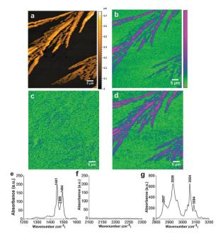
Fig. 3 (a) Topographic image of photosynthesized PDPB by conventional AFM. AFM-IR mappings of the photo-induced PDPB polymer nanostructures synthesized in a swollen hexagonal phase with  $\phi=2.21$ ,  $C_{\rm s}=0.3$  mol L $^{-1}$  measured at different fixed wavenumbers: 1490 cm $^{-1}$  (b), 2146 cm $^{-1}$  (c) and 3054 cm $^{-1}$  (d). (e–g) nanoIR spectra recorded at three different spectral regions of the PDPB polymer.
