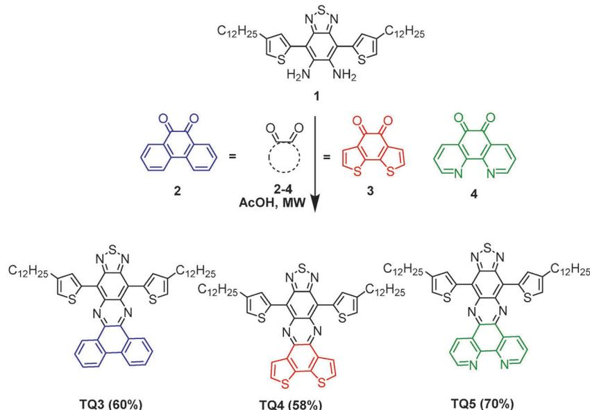
Scheme 2 Synthesis of the fused-ring TQ derivatives TQ3–TQ5.
