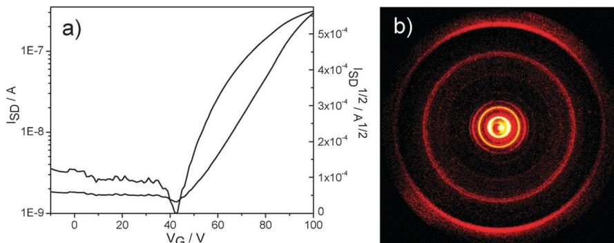
Fig. 4 (a) Transistor transfer plot and (b) 2DWAXS at 100 °C of TQ5.
