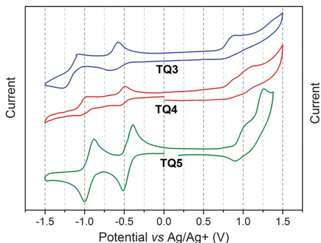
Fig. 2 Cyclic voltammograms of compounds **TQ3**–**TQ5** in DCM at 50  $\text{mV s}^{-1}$ , 0.1 M of *n*- $\text{Bu}_4\text{NPF}_6$ , glassy carbon electrode, mV vs. Ag/Ag<sup>+</sup>.
