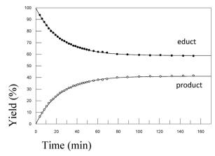
Fig. 10 Kinetics of the reaction of 1 (10 mM) and 2-phenylethanethiol (10 mM) upon dissolution in d<sub>4</sub>-MeOD. The experimental data were extracted from <sup>1</sup>H-NMR spectra (27 °C, 400.13 MHz) in which the NCH<sub>3</sub> resonance signals of 1 served as the probe
