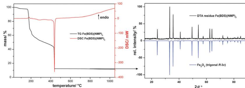
Fig. 6 Thermal decomposition of  $\text{Fe}(\text{BDS})(\text{NMP})_3$ . The DSC/TG diagram (left) shows that after desolvation there is no significant plateau. After decomposition of the desolvated sulfonates, the oxide  $\text{Fe}_2\text{O}_3$  is obtained (X-ray powder pattern shown right). The DSC/TG measurements were performed under oxygen flow.
