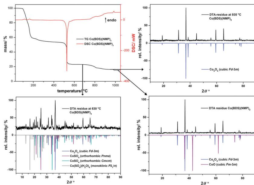
Fig. 7 Thermal decomposition of  $\text{Co}(\text{BDS})(\text{NMP})_3$ . The DSC/TG diagram (upper part, left) shows that the compound decomposes after desolvation in three steps. Firstly,  $\text{Co}_3\text{O}_4$  is formed along with some amounts of  $\text{CoSO}_4$  (lower part, left). In a further step, the latter is transformed to  $\text{Co}_3\text{O}_4$  (upper part, right), which finally starts to decompose to  $\text{CoO}$  (lower part, right).
