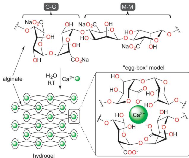
Fig. 1 Structure of the repeating units of sodium alginate ( $pK_a$  of carboxylic groups  $\sim 3$  to 4), and formation of the hydrogel by coordination of  $Ca^{2+}$  cations between adjacent alginate chains as per the "egg-box" model.
