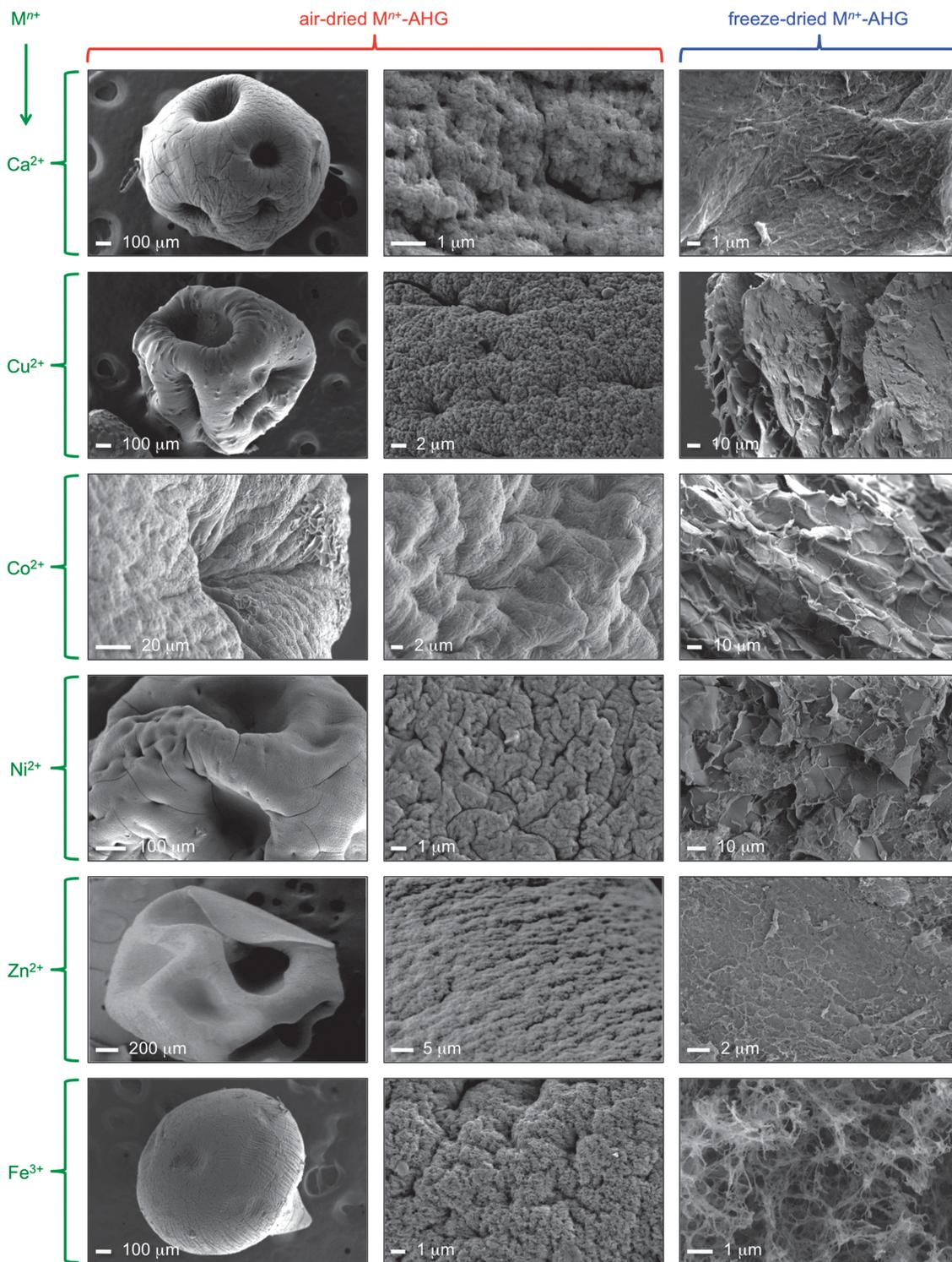
Fig. 3 SEM images of different  $M^{n+}$ -alginate-based xerogel materials. Pictures in the same row correspond to the same metal (left). Xerogels were obtained after either air-drying (left and middle columns) or freeze-drying (right column) the corresponding  $M^{n+}$ -AHG beads.
