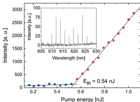
**Fig. 3** Input–output curve of a WGM microgoblet laser emitting at  $\lambda = 623.7$  nm. The lasing threshold upon excitation with a green laser diode is 0.54 nJ in air. Data points below and above threshold are marked in blue and red, respectively. The inset shows a typical multimode emission spectrum of the investigated microgoblet laser when pumped well above the lasing threshold.
