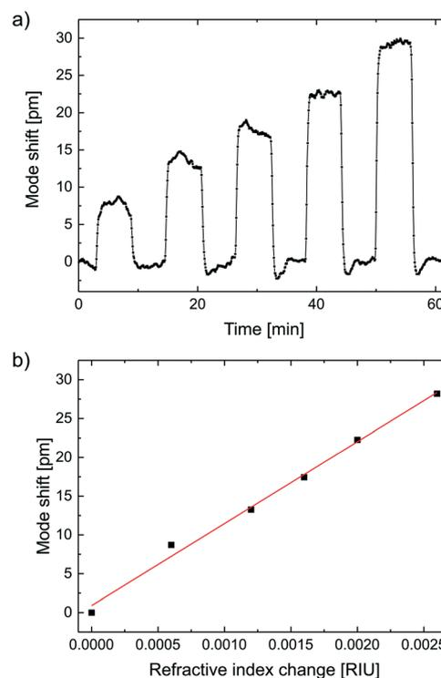
**Fig. 5** (a) Spectral shifts of a microgoblet laser mode upon injection of glycerol–water solutions with increasing refractive indexes of 1.3335 to 1.3355. Between subsequent injections of high-index solutions, deionized water with a refractive index of 1.3329 was injected for referencing. (b) A bulk refractive index sensitivity of 10.56 nm per RIU was calculated from the linear fit (red) applied to the data.
