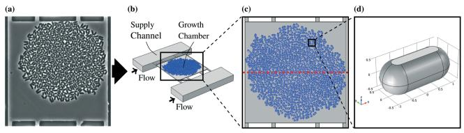
Fig. 1 (a) Microscopic picture of a real colony in a chamber, (b) three-dimensional representation of one growth chamber with cell colony (in blue) and adjacent supply channels, (c) large colony model as a whole, the red dash dotted line indicates the plane of symmetry, (d) single cell model, the flat space shows where the cell is in direct contact with the chamber ceiling.
