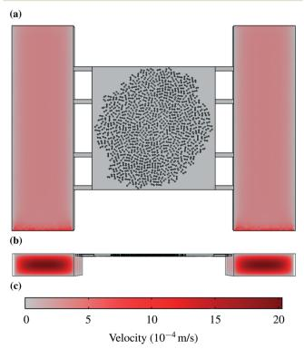
Fig. 2 Velocity profiles: (a) Liquid velocity halfway between the bottom and the top of the chamber. (b) Velocity profiles in the supply channels. (c) Scale for velocities in  $m s^{-1}$ .
