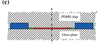
Fig. 7 Basic geometry of a lab-on-a-chip device. (a) Shows a complete cell array, (b) a single chamber from above and (c) a side view with the position of PDMS chip and glass plate indicated. The dash dotted line shows the line of symmetry.
