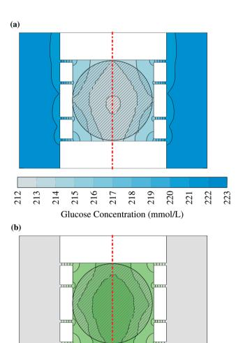
Fig. 3 Glucose (a) and lactic acid (b) concentrations in picoliter bioreactor. The striped area indicates the position of the bacterial colony, while the dash dotted line shows plane of symmetry. The cells have been omitted from this picture. The flow enters the supply channels from the lower end of the figure.
