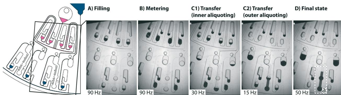
**Fig. 4** Experiment showing principle of centrifugo-pneumatic multi-liquid aliquoting with stained sample material. Labels A)–D) describe the fluidic state of the inner and outer aliquoting as detailed in the caption of Fig. 2. Every second collection chamber is combined with a quantification structure (a) for measurement of aliquoted volumes. The quantification structure is described in detail in Fig. 5.
