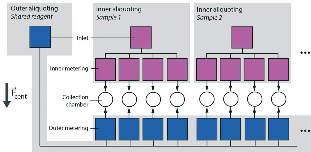
**Fig. 1** The process chain of centrifugo-pneumatic multi-liquid aliquoting consists of the unit operations inner and outer aliquoting. Each aliquoting structure comprises an inlet and multiple metering chambers connected to the inlet. Each aliquot from the outer aliquoting is combined with a complementary aliquot from the inner aliquoting within a collection chamber. The principle of the metering structures to be implemented in centrifugal microfluidics is depicted in Fig. 2.
