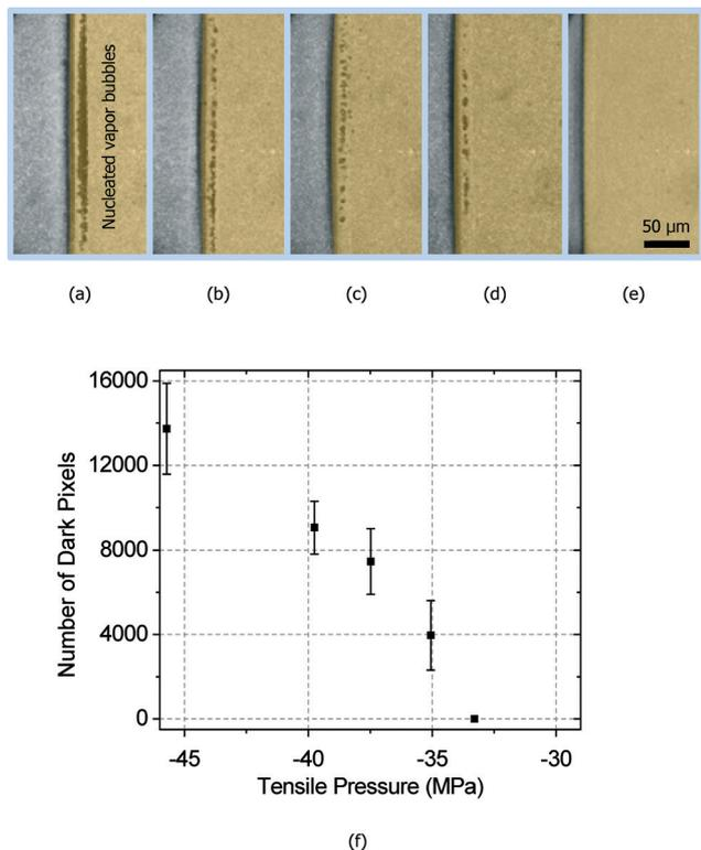
Fig. 5 Images of homogeneous nucleation with various standoff distances of (a) 220.7, (b) 231.0, (c) 242.4, (d) 252.0 and (e) 260.2  $\mu\text{m}$ . (f) Number of dark pixels in the nucleation region as a function of the tensile pressure.
