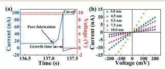
Fig. 2 (a) Leakage current through the  $SiN_x$  membrane a few seconds before nanopore fabrication by CBD at 10 V. The instant of nanopore fabrication is characterized by a sudden increase in current. (b) Current–voltage (*I–V*) curves used to infer nanopore diameter using a conductance-based model for 5 independently fabricated nanopores on a single five-channel device.
