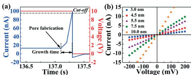
Fig. 2 (a) Leakage current through the SiN<sub>x</sub> membrane a few seconds before nanopore fabrication by CBD at 10 V. The instant of nanopore fabrication is characterized by a sudden increase in current. (b) Current–voltage ( $I$ – $V$ ) curves used to infer nanopore diameter using a conductance-based model for 5 independently fabricated nanopores on a single five-channel device.
