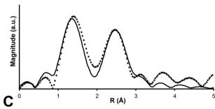
Fig. 5 Mn EXAFS. Three panel results of EXAFS analysis of Mn within the fossil specimen. (A) Raw data for the absorption coefficient measurement at the Mn K-edge. (B) EXAFS function presented for the specimen (solid line) and a computed fit to the data (dashed line). (C) Fourier transform of EXAFS where the data are presented as the discrete points and the best fit is shown as the thin solid line. Clearly the RDF shows two strong backscattering shell surrounding the central Mn absorber.
