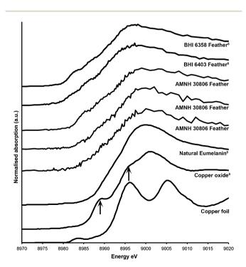
Fig. 4 Copper XANES spectra. Cu XANES spectra are from a copper standard (copper foil) and three different feathers from AMNH FARB 30806. The spectra from these have been plotted along with published spectra from copper oxide, natural copper eumelanin, and two isolated feathers from the Green River Formation (BHI 6358 and 6403).8 The arrows on the copper oxide are pointing to peaks that are unique to that spectrum and do not occur in the fossil material.
