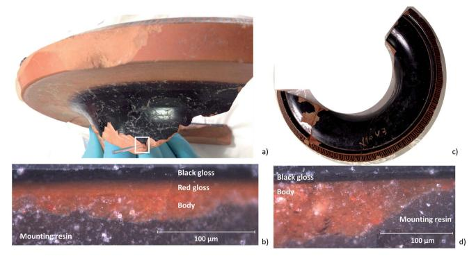
Fig. 1 (a) Sampling point of JPGM 81.AE.206.d.2005\_ext. (b) Cross-section of sample JPGM 81.AE.206.d.2005\_ext. From top: black gloss, red gloss, body. (c) Sampling point of JPGM 81.AE.206.d.2005\_int. (d) Cross-section of sample JPGM 81.AE.206.d.2005\_int. From top: black gloss, body.
