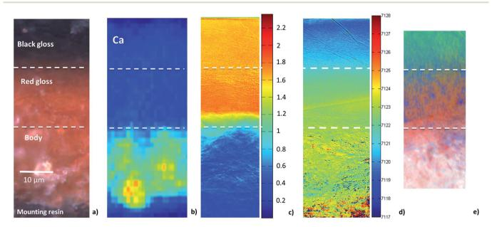
Fig. 4 (a) Cross-section of sample EXT. (b) Ca XRF map. (c) X-ray absorption image at 7080 eV showing different porosity in the two glosses compared to the body. (d) Fe-edge position map. (e) RGB phase map generated by the fit of single pixel XANES spectra with iron oxide standards. The phase map shows that the black gloss is composed of hercynite (green), the red gloss of hematite (red) and the body of a mixture of maghemite (blue) and hematite.
