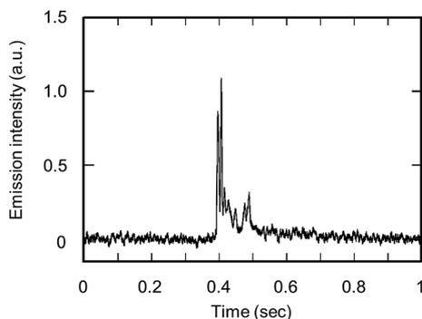
**Fig. 8** Emission intensities of Na I 588.99 nm from a single droplet containing 3300 yeast cells. Emission intensities were observed by side-on observation (RF power, 700 W; carrier gas flow, 0.4  $\text{L min}^{-1}$ ; droplet volume, 15 nL (300  $\mu\text{m}$ )).
