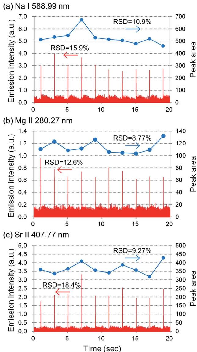
Fig. 7 Emission profiles of (a) Na I 588.99 nm, (b) Mg II 280.27 nm, and (c) Sr II 407.77 nm, with injection of a series of droplets generated from  $10 \mu\text{g mL}^{-1}$  Na, Mg and Sr standard solution. Emission intensities were observed by side-on observation (RF power, 700 W; carrier gas flow,  $0.4 \text{ L min}^{-1}$ ; droplet volume, 15 nL ( $300 \mu\text{m}$ ); droplet introduction frequency, 0.5 Hz).
