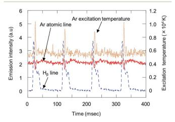
Fig. 4 Emission profiles of the Ar atomic line (Ar I 425.11 nm),  $H_{\beta}$  line (486.13 nm) and Ar excitation temperature with injection of droplets generated from ultra-pure water. Emission intensities were observed by side-on observation (RF power, 1000 W; droplet volume, 5.5 nL (220  $\mu$ m); droplet introduction frequency, 10 Hz).
