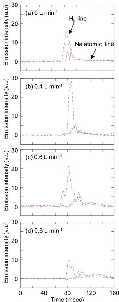
Fig. 6 Variation in emission profiles of the Na atomic line (Na I 588.99 nm) and  $H_{\beta}$  line (486.13 nm) with a carrier gas flow of (a)  $0 \text{ L min}^{-1}$ , (b)  $0.4 \text{ L min}^{-1}$ , (c)  $0.6 \text{ L min}^{-1}$ , and (d)  $0.8 \text{ L min}^{-1}$ , with injection of droplets generated from  $10 \mu\text{g mL}^{-1}$  Na standard solution. Emission intensities were observed by end-on observation (RF power, 700 W; droplet volume, 4.7 nL ( $210 \mu\text{m}$ )).
