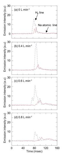
Fig. 6 Variation in emission profiles of the Na atomic line (Na I 588.99 nm) and  $H_{\beta}$  line (486.13 nm) with a carrier gas flow of (a) 0 L min $^{-1}$ , (b) 0.4 L min $^{-1}$ , (c) 0.6 L min $^{-1}$ , and (d) 0.8 L min $^{-1}$ , with injection of droplets generated from 10  $\mu g$  mL $^{-1}$  Na standard solution. Emission intensities were observed by end-on observation (RF power, 700 W; droplet volume, 4.7 nL (210  $\mu m$ )).
