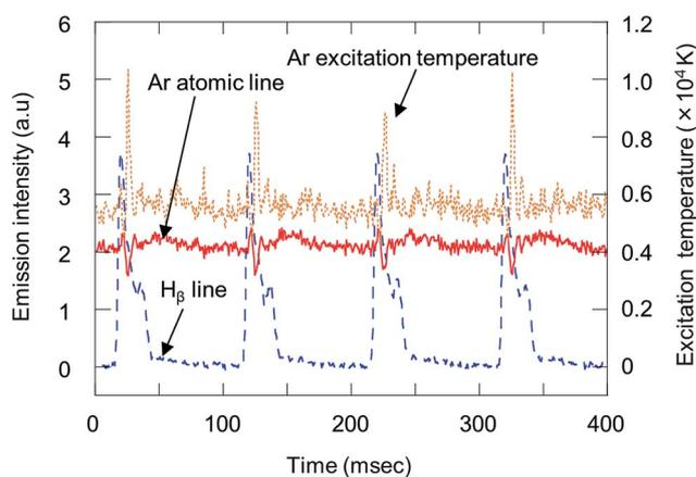
Fig. 4 Emission profiles of the Ar atomic line (Ar I 425.11 nm),  $\text{H}_\beta$  line ( $486.13\text{ nm}$ ) and Ar excitation temperature with injection of droplets generated from ultra-pure water. Emission intensities were observed by side-on observation (RF power,  $1000\text{ W}$ ; droplet volume,  $5.5\text{ nL}$  ( $220\text{ }\mu\text{m}$ ); droplet introduction frequency,  $10\text{ Hz}$ ).
