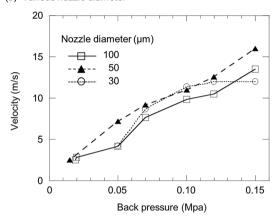
Fig. 3 Droplet velocity as a function of back pressure at (a) various valve open times: 0.5, 1.0 and 10 ms and (b) various nozzle diameters: 30, 50 and 100  $\mu$ m.
