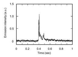
Fig. 8 Emission intensities of Na I 588.99 nm from a single droplet containing 3300 yeast cells. Emission intensities were observed by side-on observation (RF power, 700 W; carrier gas flow, 0.4 L min $^{-1}$ ; droplet volume, 15 nL (300  $\mu$ m)).
