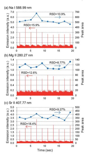
Fig. 7 Emission profiles of (a) Na I 588.99 nm, (b) Mg II 280.27 nm, and (c) Sr II 407.77 nm, with injection of a series of droplets generated from 10  $\mu g$  mL  $^{-1}$  Na, Mg and Sr standard solution. Emission intensities were observed by side-on observation (RF power, 700 W; carrier gas flow, 0.4 L min $^{-1}$ ; droplet volume, 15 nL (300  $\mu$ m); droplet introduction frequency, 0.5 Hz).
