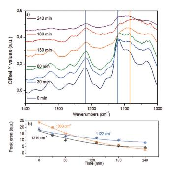
Fig. 7 (a) ATR-IR spectra in the spectral region of 1400–1000 cm<sup>-1</sup> for organosolv lignin reacting over Ni/HBEA in n-hexadecane at 523 K and 20 bar H<sub>2</sub>. (b) Deconvoluted and integrated peak areas at 1219 cm<sup>-1</sup>, 1122 cm<sup>-1</sup> and 1080 cm<sup>-1</sup> representing the aromatic C-C-O stretching vibration, the aliphatic secondary and primary C-C-O stretching vibrations, respectively.
