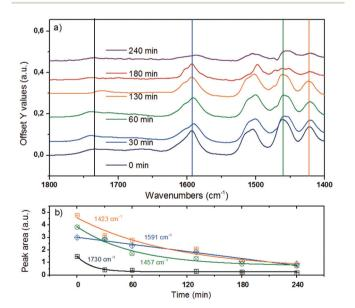
**Fig. 6** (a) ATR-IR spectra in the spectral region of  $1800-1300~\rm cm^{-1}$  for organosolv lignin reacting over Ni/HBEA in n-hexadecane at 523 K and 20 bar  $H_2$ . (b) Qualitative trend for peak areas at 1730 cm $^{-1}$  for C=O stretching vibration, 1591 cm $^{-1}$  for symmetric aryl ring stretch, 1457 cm $^{-1}$  for CH $_3$ -O bend and 1423 cm $^{-1}$  for aromatic skeletal vibration.  $^{43,44,52}$
