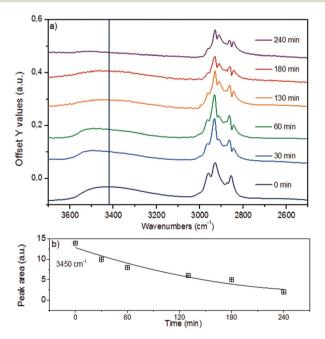
Fig. 5 (a) ATR-IR spectra in the spectral region of  $3800-2500~\rm cm^{-1}$  (O–H and C–H stretching vibrations) for organosolv lignin reacting over Ni/HBEA in n-hexadecane at 523 K and 20 bar  $H_2$ . (b) The evolution of integrated peak area at 3430 cm $^{-1}$ , representing the O–H stretching vibration, as a function of reaction time.
