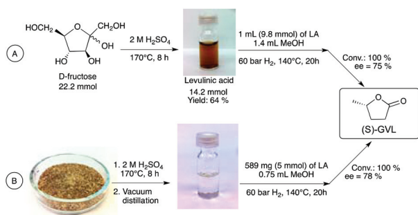
Scheme 3 Conversion of D-fructose (A) and mixed biomass waste (B) to (S)-GVL.
