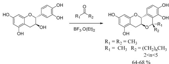
Fig. 21 Oxa-Pictet-Spengler reaction of catechin and various ketones.
