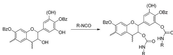
**Fig. 36** Reaction between partially benzoylated mimosa tannins and isocyanates.
