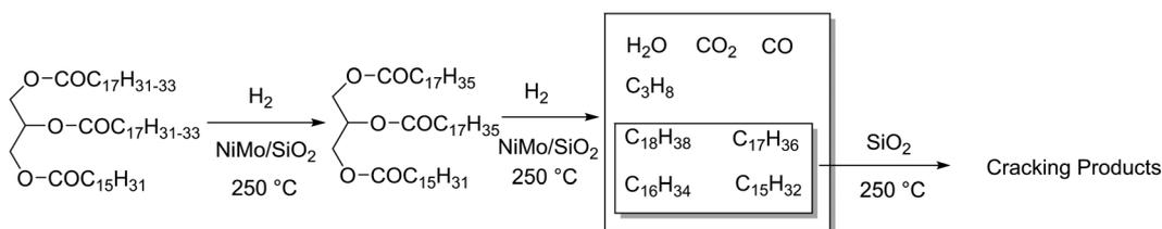
Fig. 12 NiMo catalysed hydrotreatment of *Jatropha* oil to C<sub>18–15</sub> alkanes and subsequent cracking products.
