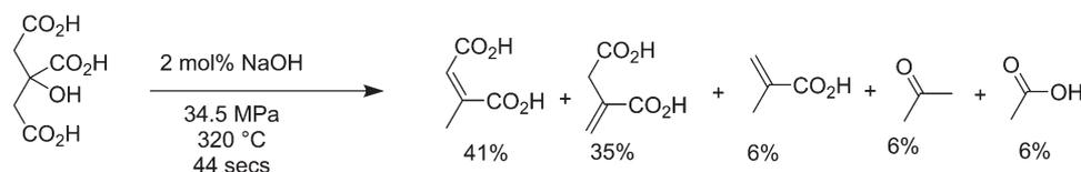
Fig. 13 High temperature water decarboxylation of citric acid.
