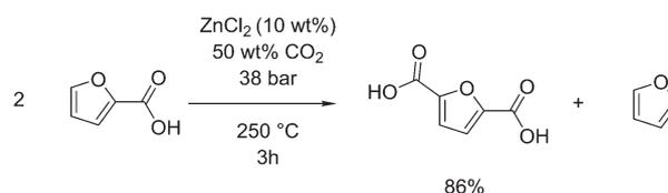
Fig. 8 Henkel reaction performed on furoic acid.
