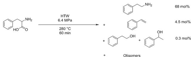
Fig. 14 Degradation of phenylalanine in HTW conditions.
